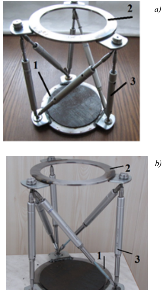
Figure 1. Manipulators of platform robots parallel manipulators have a large bearing capacity as their upper platform can be rigidly connected with the float. In these models (Fig. 1), the lower platform 1 is connected to the upper platform 2 by means of six actuators 3. The models differ by the actuators interconnection schemes.
