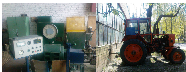
Fig. 1. Equipment for determining the operational characteristics of the diesel engine KI-5543-GOSNITI
