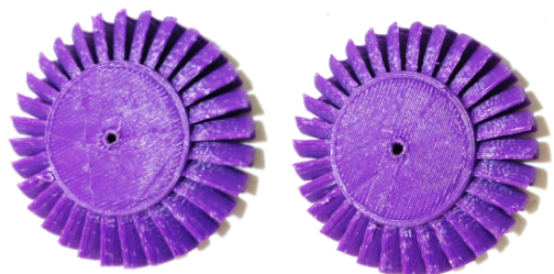
Fig. 4 Three-dimensional printed models of Impulses turbine Dia. 48 and 50 mm with the variation of the number of blades.
