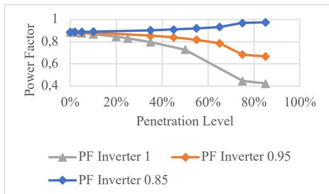
**Fig. 14.** System Power Factor under different PV Power Factor
