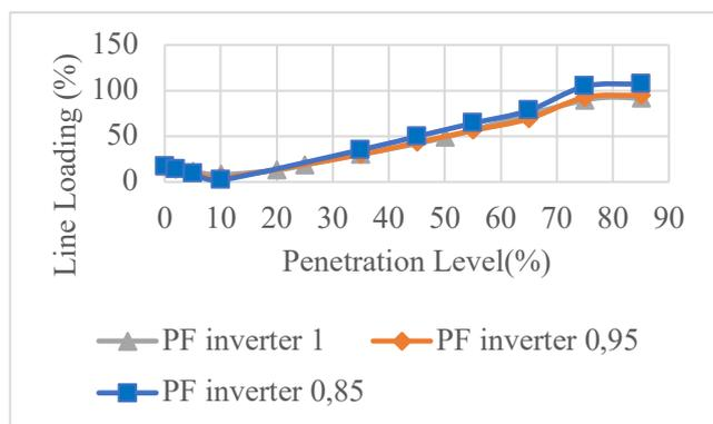
**Fig. 13.** Line Loading Profiles under different PV Power Factor
