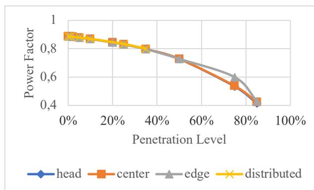
Fig. 11. System Power Factor under different Scenario
