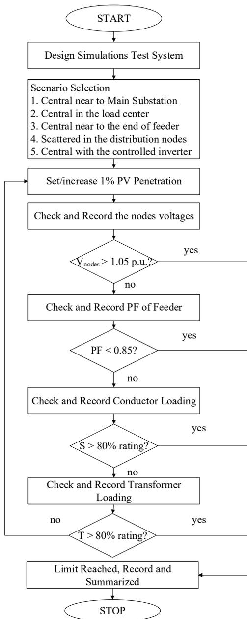
Fig. 4. Procedure for determining the PV Hosting Capacity
