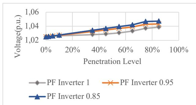
**Fig. 12.** Obtained Operating Voltage under different PV Power Factor
