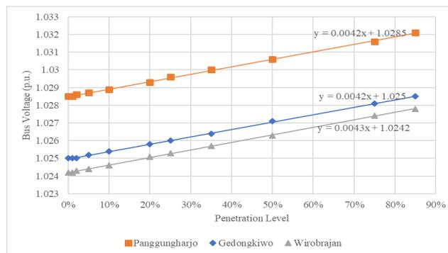
Fig. 6. Obtained Operating Voltage at Buses in Head Scenario
