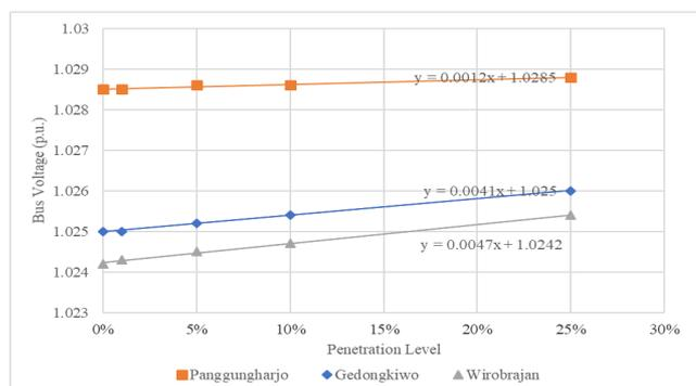
Fig. 9. Obtained Operating Voltage at Buses in Distributed Scenario
