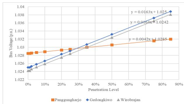
Fig. 7. Obtained Operating Voltage at Buses in Center Scenario
