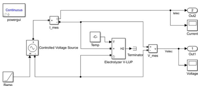
**Fig. 7.** Circuit to obtain polarization curves in Matlab/Simulink
