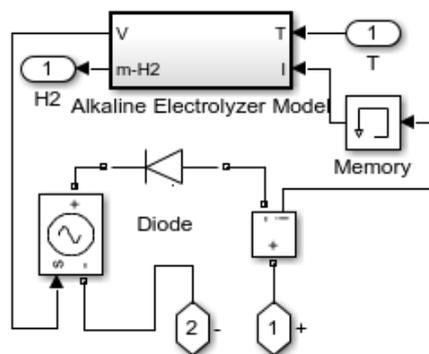
Fig. 1. Electrolyser simscape power systems block [15].
