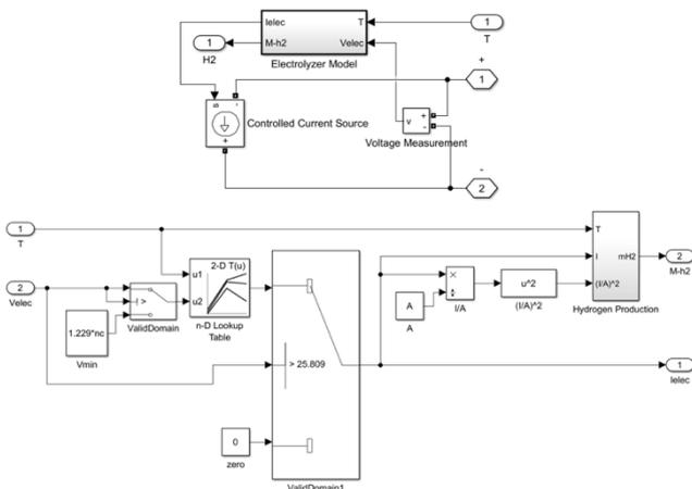
Fig. 5. Implementation of the New representation in Matlab/Simulink
