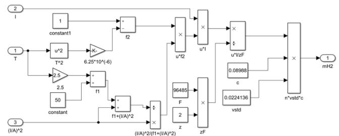
Fig. 6. Implementation of hydrogen production in Matlab/Simulink
