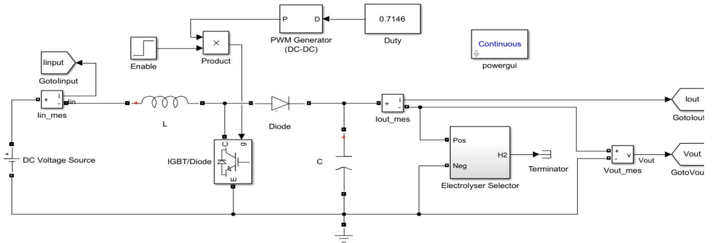
**Fig. 9.** Boost converter and electrolyser system.
