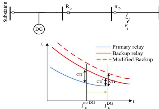
Fig. 1. Increased CTI due to DG’s contribution seen by both relays
