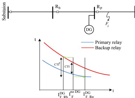
Fig. 2. Reduced CTI due to DG’s contribution seen by primary relay
