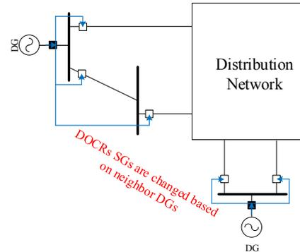
Fig. 3. Adaptive protection with SGs in some relays
