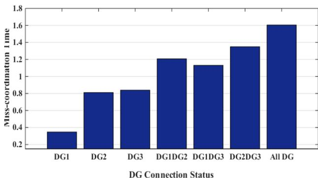
Fig. 7. Miss-coordination due to DGs penetration
