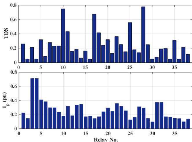
Fig. 6. Optimal settings of DOCRs for scenario 4.1
