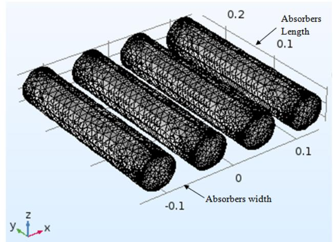
**Fig.3** Absorber tubes entire mesh.
