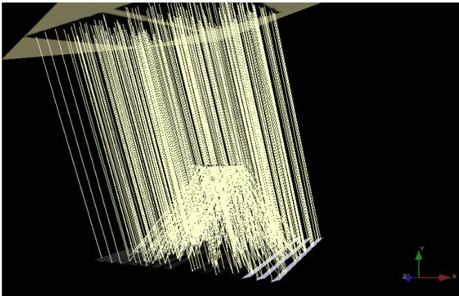
**Fig. 2** Isometric view of the ray tracing model in Tonatiuh with 500 sun rays.
