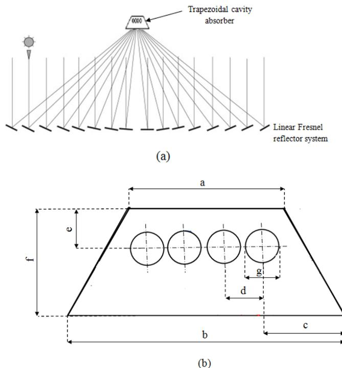
**Fig. 1.** illustrative drawing of the suggested cavity absorber for LFR system. (a) Full plant. (b) Geometry of the proposed cavity absorber.
