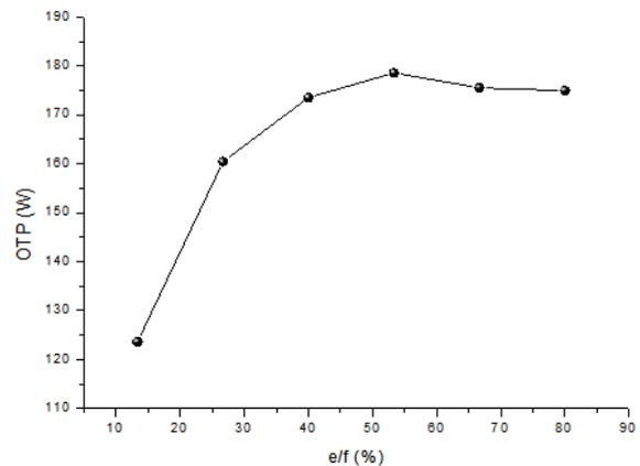
**Fig.7** The relationship between Output Thermal Power of absorber tubes and Distance between the cavity top and
