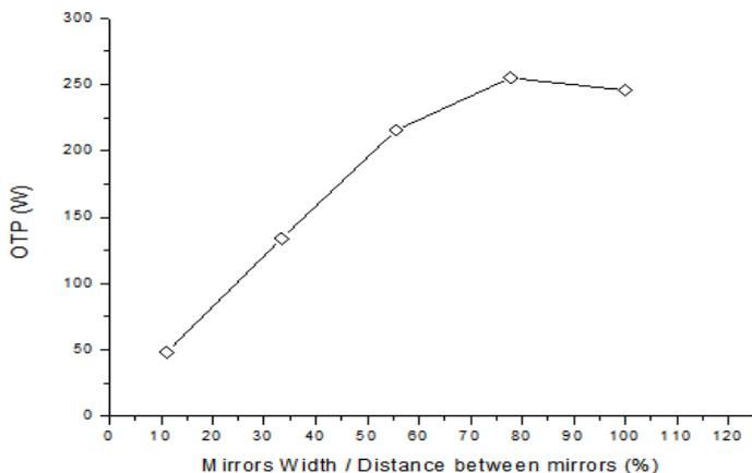
**Fig.4** The relationship between Output Thermal Power of absorber tubes and Mirrors width/Distance between mirrors.
