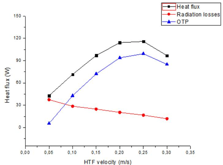
Fig.9 Heat flux, radiation losses and OTP variation in relation to HTF velocity.
