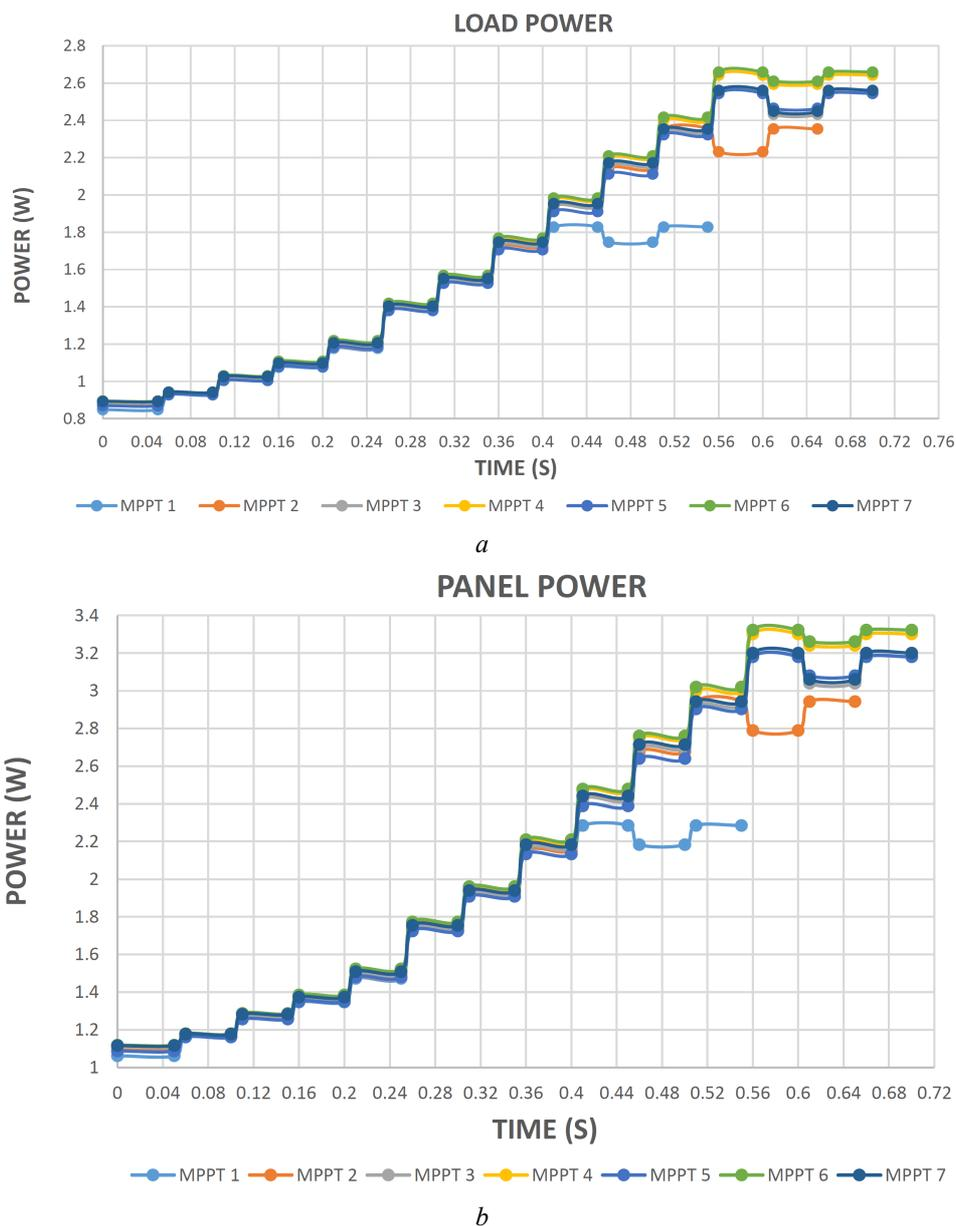
**Fig. 11.** The powers during the performance of the proposed tracking algorithm in mud/dirt condition **(a)** The load power, **(b)** The PV power
