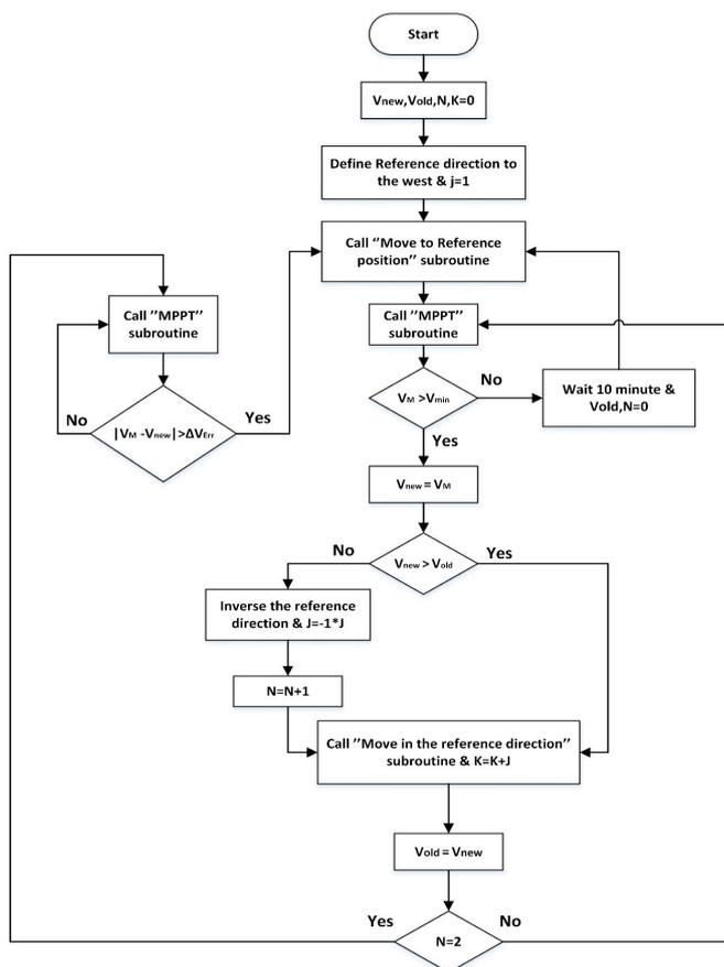
**Fig. 5.** Flow diagram of the proposed sensorless tracking method
