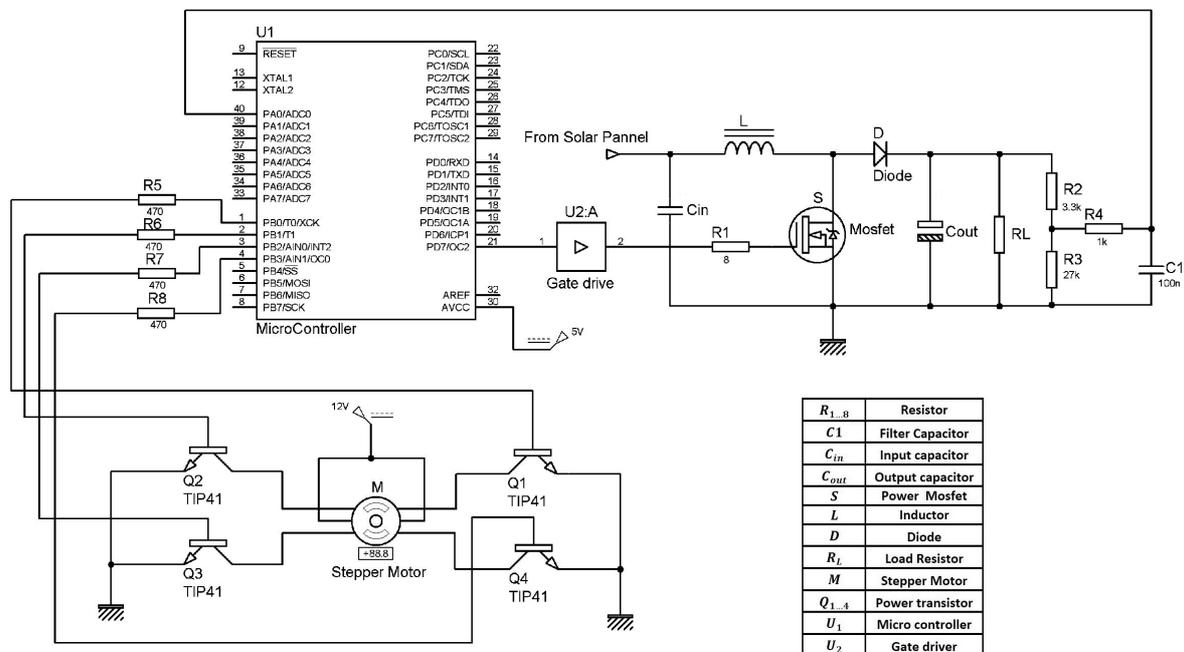
Fig. 4. Schematic diagram of the complete system
