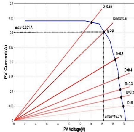
**Fig. 3.** Measured V-I characteristic of the utilized PV module
