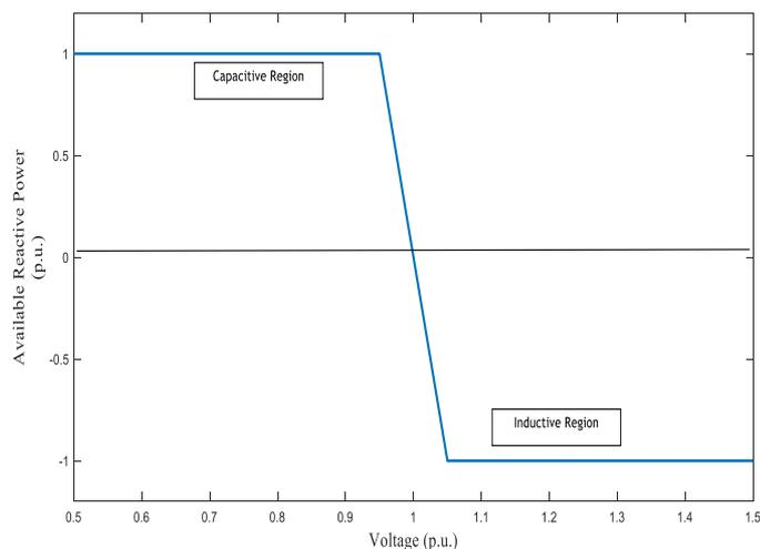
**Figure 9.** Typical Volt-VAR curve considered for study.
