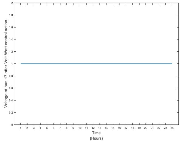
Figure 13. Voltage at bus-17 after Volt-Watt Control.
