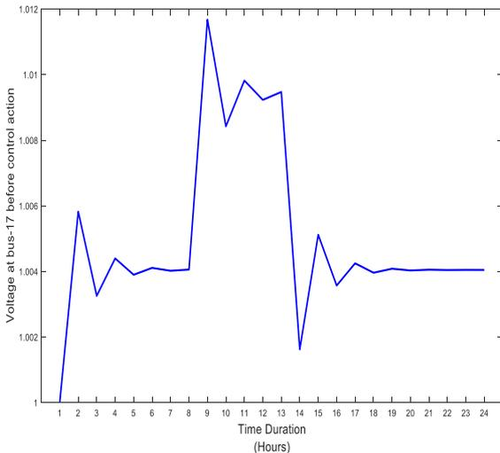
Figure 11. Voltage at bus-17 without control action.
