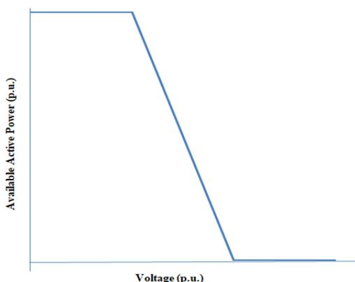
Figure 3. Typical Volt-Watt curve
