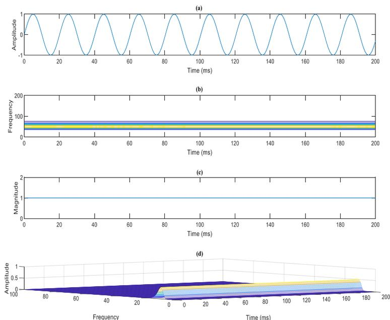
Figure 5. TFR of 1 p.u. sinusoid obtained through S-transform.
