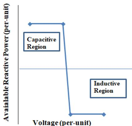
Figure 2: Typical Volt-VAr curve.
