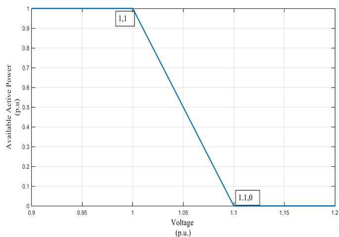
**Figure 10.** Typical Volt-Watt curve considered for study.
