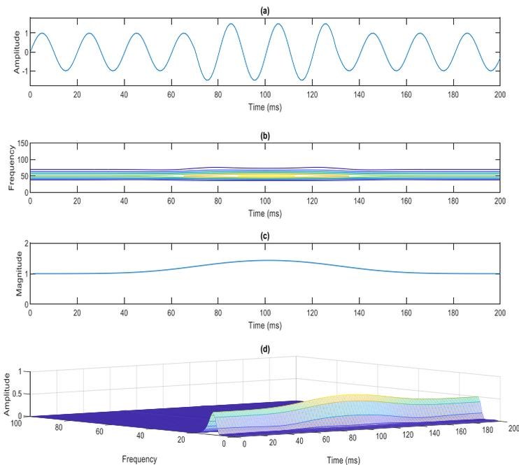
**Figure 7.** TFR of swell waveform obtained through S-transform.
