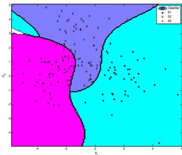
**Figure 8.** Boundary plot of LS-SVM for grouping of voltage Sag.
