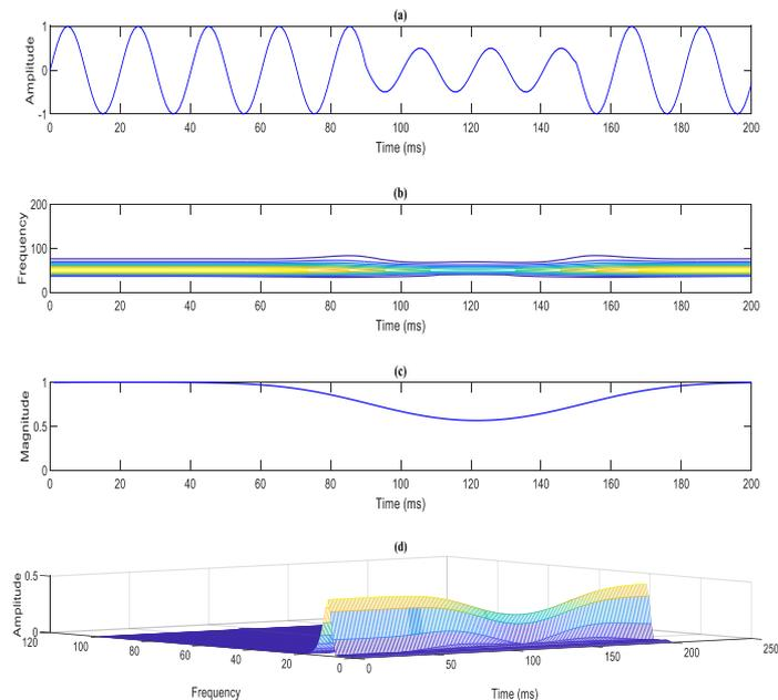
Figure 6. TFR of sag waveform obtained through S-transform.
