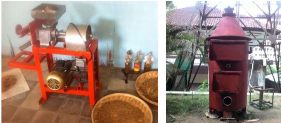
Figure 1. The OWRS devices for Giwangan traditional market in Yogyakarta. (Left) Dewatering Machine. (Right) Hookway Pyrolysis
