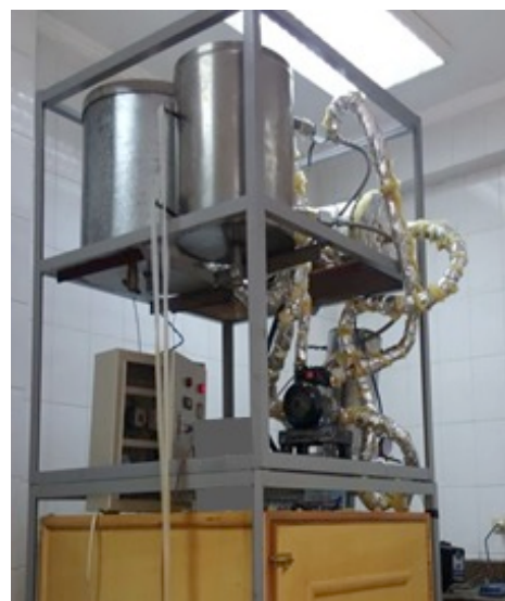
Fig. 9. A Photograph of main components of the adsorption system with the cold store.
