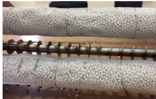
Fig. 12. Finned tubes surrounded by zeolite granules.
