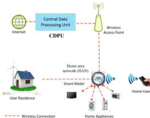
Fig.2. Smart Metering Architecture
