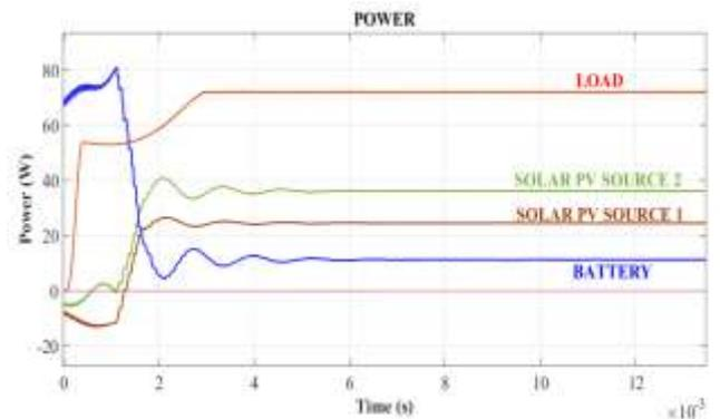
Fig. 6. Power flows in various nodes during Discharge Mode 1
