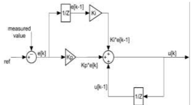
Fig. 4. Modified PI controller unit for transient minimization
