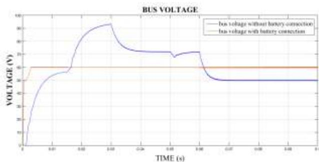
**Fig.11.** DC Bus voltage without a battery support unit connection
