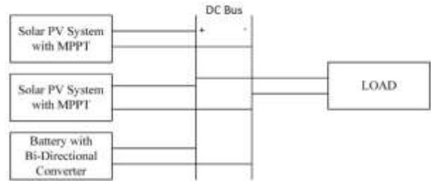
**Fig. 1.** Block Diagram of considered DC microgrid
