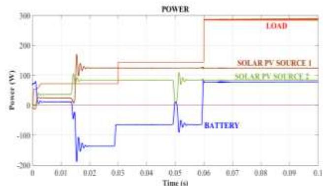
Fig.10. Power absorbed and delivered by different sources and loads.
