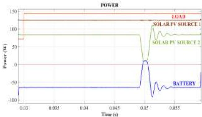
Fig. 8. Power flows in various nodes during Charging Mode 2
