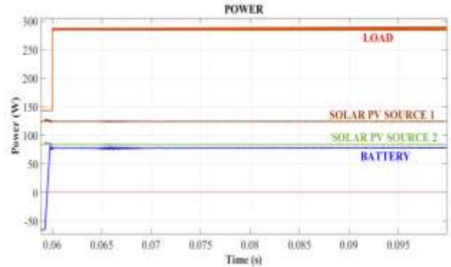
Fig. 9. Power flows in various nodes during Discharge Mode 2
