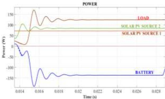
Fig. 7. Power flows in various nodes during Charging Mode 1
