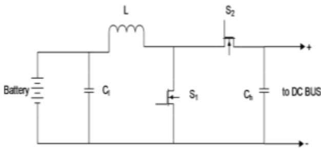
Fig. 3. Circuit diagram of Bidirectional DC-DC Converter
