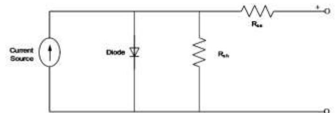
**Fig. 2.** Single Diode Model of Solar Panel
