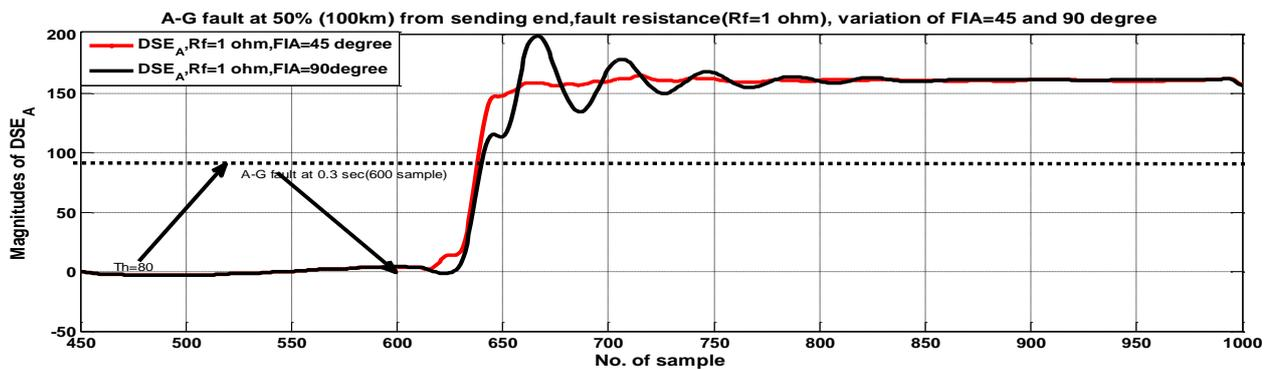
**Fig. 7.** A-Phase fault, distance 50% from B-S,  $R_f = 1\Omega$  and  $FIA = 45^\circ$  and  $90^\circ$  and wind speed=15m/sec
