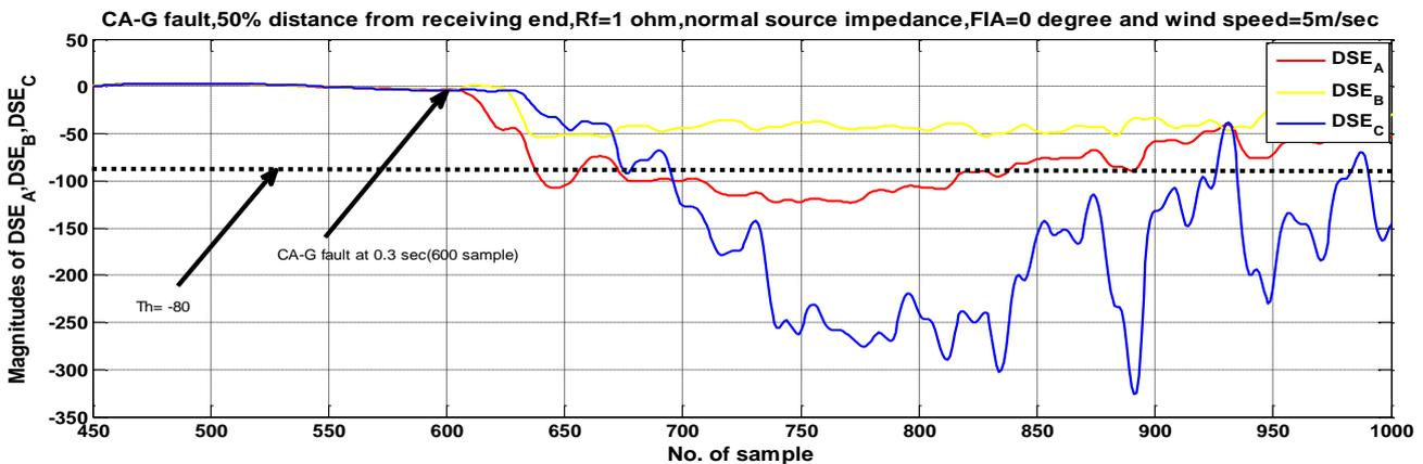
**Fig. 9(a).** CA-G fault at B-4 at 0.3 sec, distance 50% (100km) from wind farm,  $R_f=1\Omega$  normal SI,  $FIA=0^\circ$  and wind speed=5m/sec
