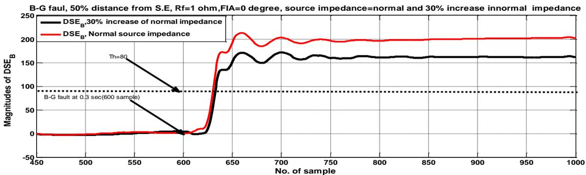
**Fig. 6(b).** A comparative study of B-G fault at 100km (50%) distance from bus B-S at 0.3 sec,  $R_f = 1\Omega$ ,  $FIA = 0^\circ$ , SI=normal SI, 30% increase of SI and wind speed=15m/sec
