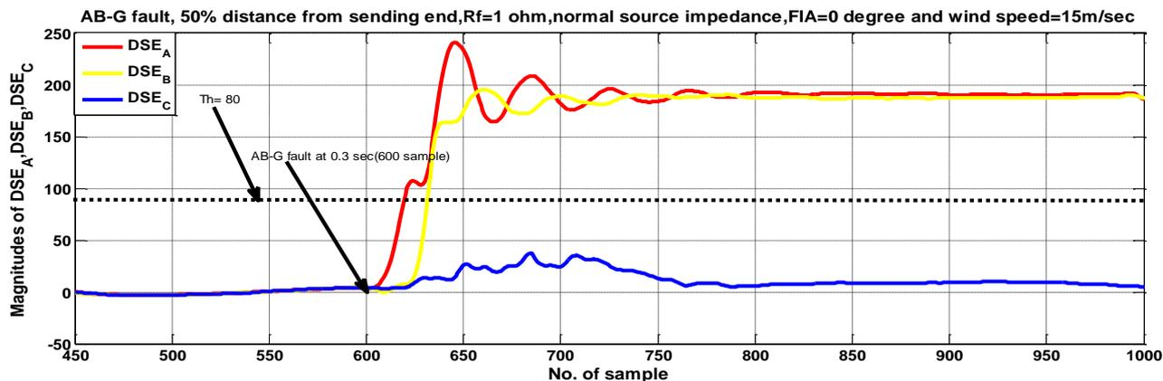
**Fig. 9(b).** AB-G fault at B-S at 0.3 sec, distance 50% (100km) from bus B-S,  $R_f = 1\Omega$  normal SI,  $FIA = 0^\circ$  and wind speed=15m/sec
