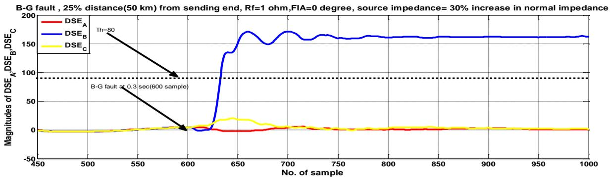
**Fig. 6(a).** B-G fault, 25% distance(50km) from sending bus(B-S) at 0.3 sec, SI = 30% increase of normal SI,  $R_f = 1\Omega$ ,  $FIA = 0^\circ$  and wind speed=15m/sec
