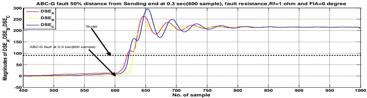
Fig. 4(a). ABC-G fault at 0.3sec from 100km distance (50% of total distance from STATCOM to sending Bus B-S), Rf=1Ω,FIA=0<sup>0</sup> and wind speed=15m/sec
