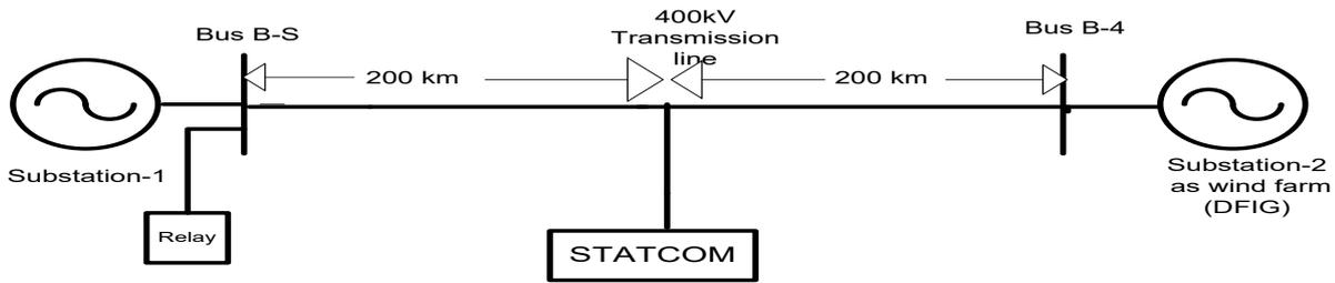
Fig. 2(b). Schematic diagram of proposed scheme
