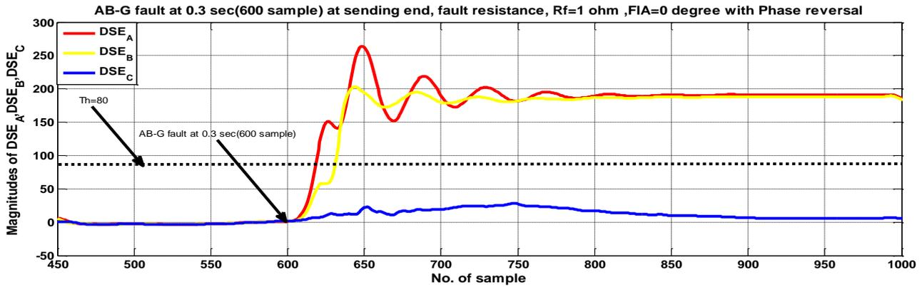
**Fig. 8.** AB-G fault at 0.3 sec, 50% distance (100km) from B-S at  $R_f=1\Omega$  and  $FIA=0^\circ$  with phase reversal, wind speed=15m/sec
