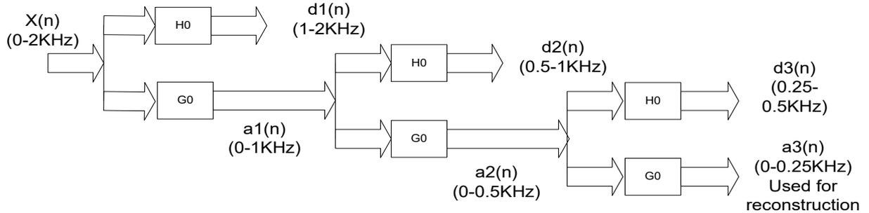
Fig. 1. Three stage wavelet decomposition tree
