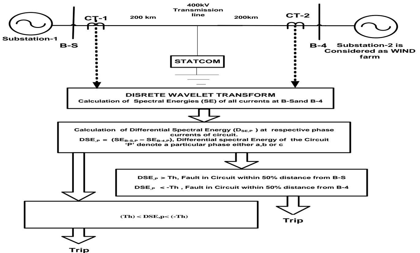
Fig. 3. Proposed relaying scheme
