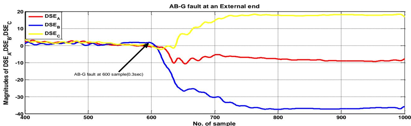
**Fig. 10.** AB-G fault at 0.3 sec at an external end at  $R_f = 1\Omega$  and  $FIA = 0^\circ$ , wind speed=15m/sec
