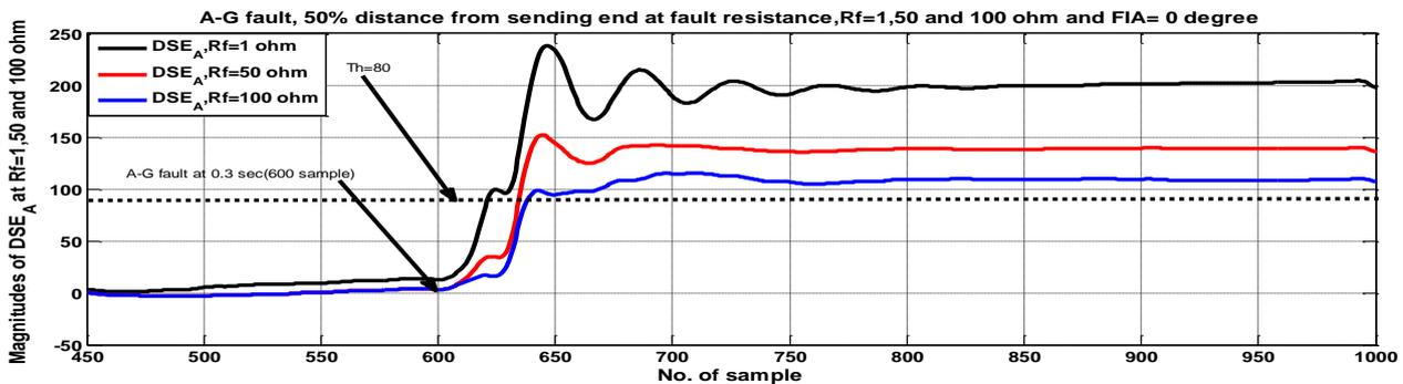
**Fig. 5.** A-G fault at 0.3 sec from B-S, fault at 100km (50%) distance from bus B-S at different values of  $R_f = 1\Omega, 50\Omega$  and  $100\Omega$ ,  $FIA = 0^\circ$  and wind speed = 15m/sec.
