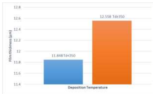
Fig. 7. Calculated film thickness of the aged (one week) NiO films at different deposition temperature.
