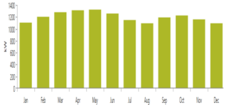
Fig. 12. Average monthly electricity generation from PV with Battery system
