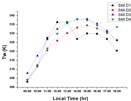
Figure 8: Hourly variation of basin water temperatures.
