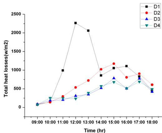
**Figure 6:** Hourly Computed total heat losses of the stills.
