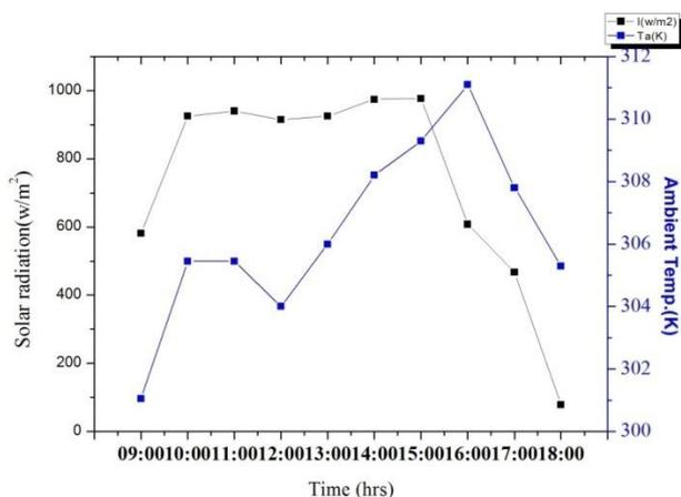
**Figure 3:** Graphs of solar radiation and ambient temperature versus local time
