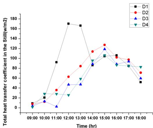
**Figure 12:** Variation of total heat transfer coefficient of the stills with day time.
