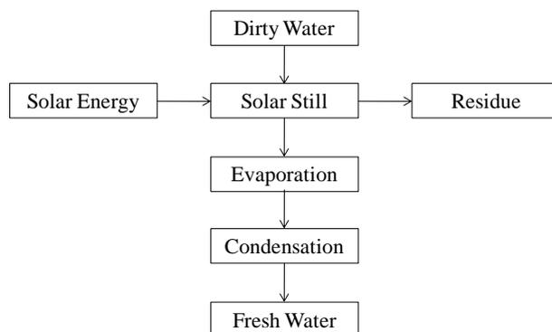
Figure 1: Schematic of Solar Distillation Process.
