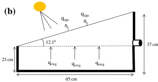
**Figure 2:** Schematic diagram of (a) conventional (b) modified solar stills
