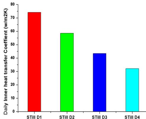
**Figure 13:** Daily total inner heat transfer coefficient of the still.
