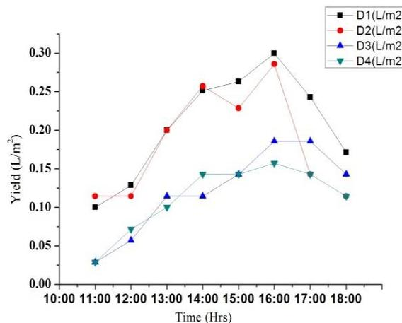
Figure 9: Variation of hourly distillate of solar stills with time.
