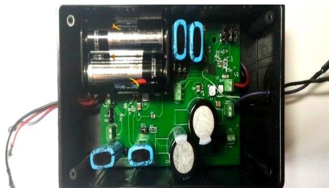
Fig. 22. Final structure of realized harvesting board for WSN node power-supply.
