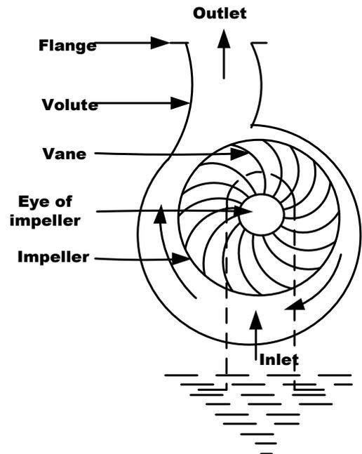
Fig. 3. Cross sectional view of centrifugal pump.
