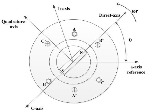
Fig. 2. PMSM in d-q axes reference frame
