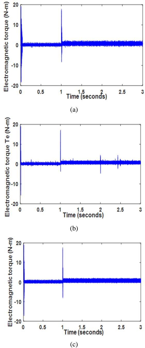
**Fig. 14.** Electromagnetic torque developed in motor (a) Conventional DTC (b) DTC – FLC (c) DTC – ANFIS.
