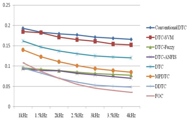
**Fig. 21.** Torque ripple for all proposed and existing DTC topologies at 500 rpm.
