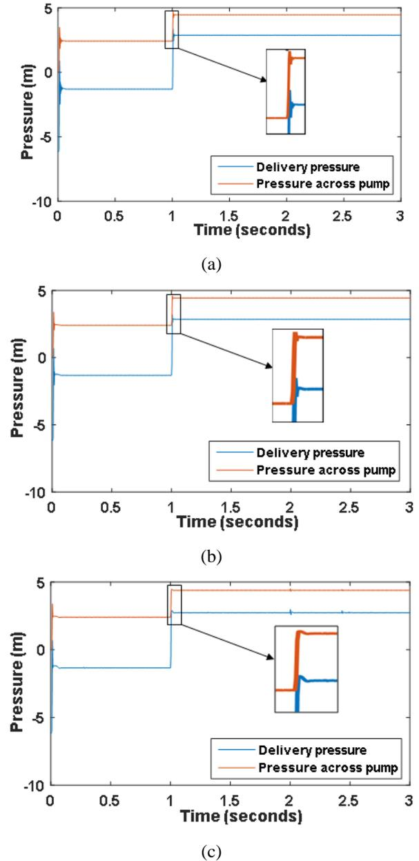
**Fig. 12.** Pump output pressure (a) Conventional DTC (b) DTC – FLC (c) DTC – ANFIS.
