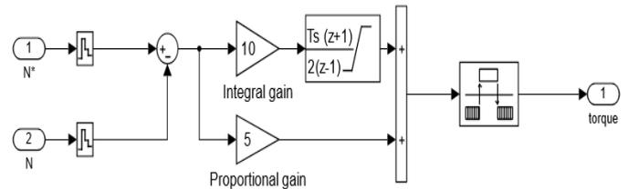
Fig. 8. Speed control with PI controller.
