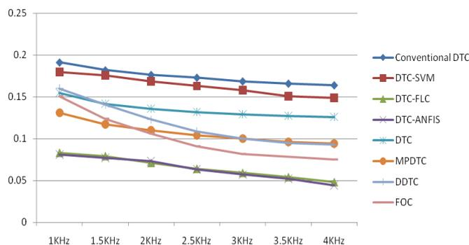
**Fig. 22.** Torque ripple for proposed and existing DTC strategies at 1000 rpm.
