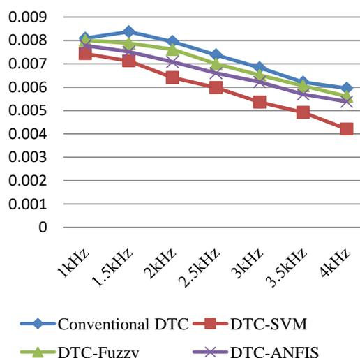
**Fig. 23.** Flux ripple for the proposed DTC strategies at 500 rpm.
