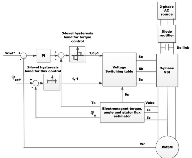
Fig. 4. Basic block diagram of DTC-traditional control
