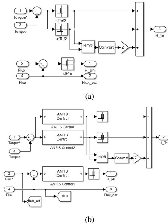
Fig. 9. Torque and flux controller (a) Conventional DTC (b) DTC with ANFIS.
