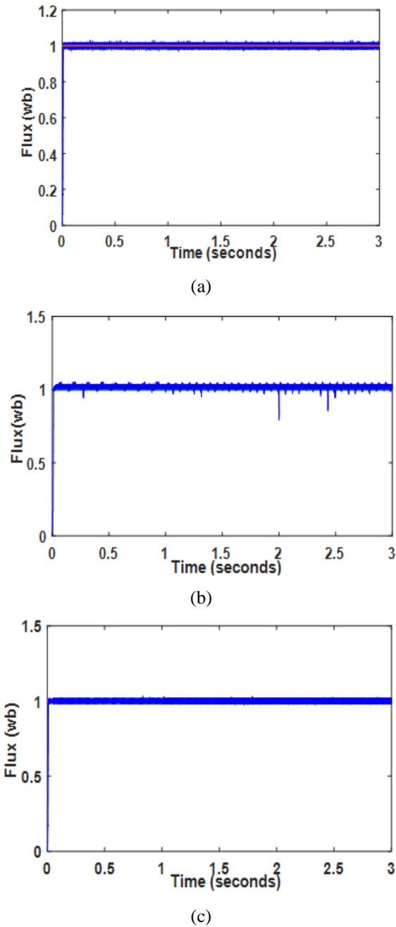
**Fig. 13.** Stator flux of PMSM (a) Conventional DTC (b) DTC – FLC (c) DTC – ANFIS
