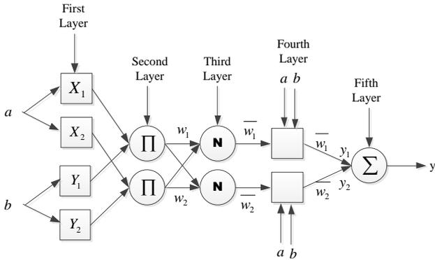
Fig. 6. ANFIS model with 2 inputs (a and b) and 1 output(y)
