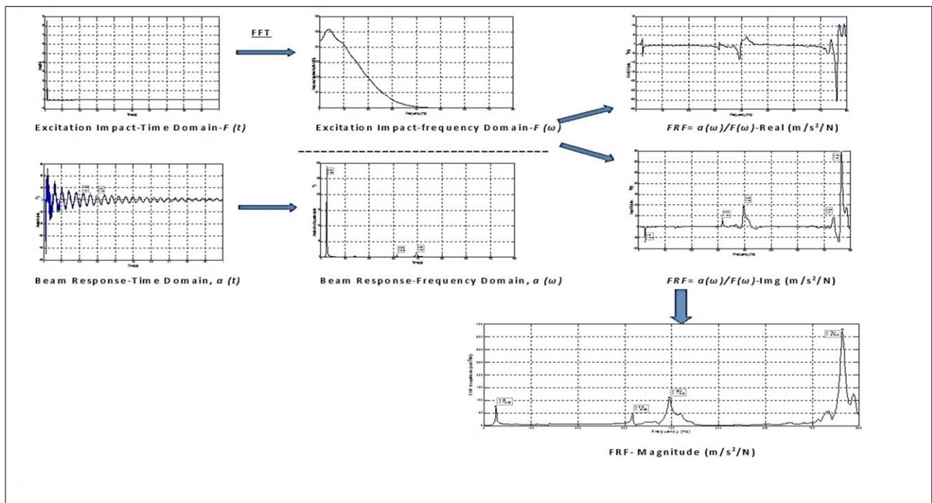
Fig. 5. The FRF computational procedure
