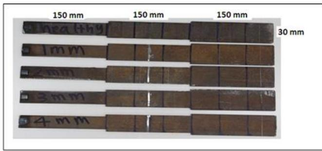
Fig. 3. The Fabricated Stepped Beams with Different Fault Size.
