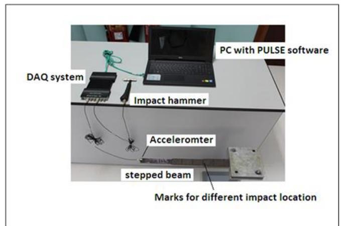
Fig. 2. The Impact Hammer Test Experimental Setup.
