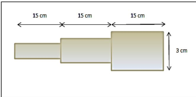
Fig. 1-b. The simplified profile (stepped beam).
