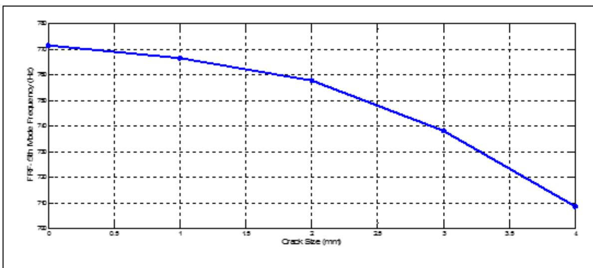
**Fig. 7.** The 5th FRF mode frequency with different fault size
