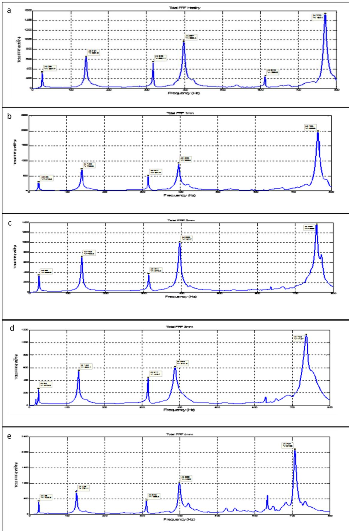
**Fig. 6.** The total averaged FRF for stepped beam with different fault size: (a) Healthy, (b) 1mm, (c) 2mm (d) 3mm and (e) 4mm.
