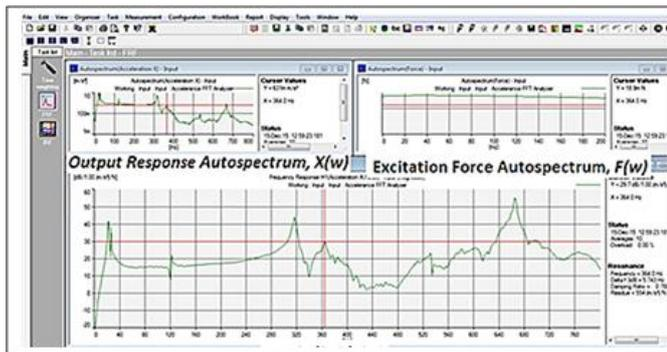
Fig. 4. The calculation of FRF of the beam with PULSE software.
