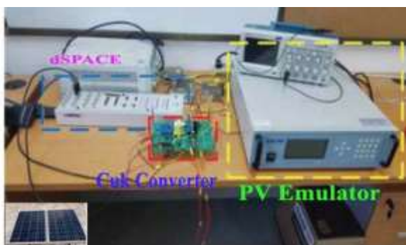
Fig. 14. Experimental developed GA based MPPT system using dSPACE control board
