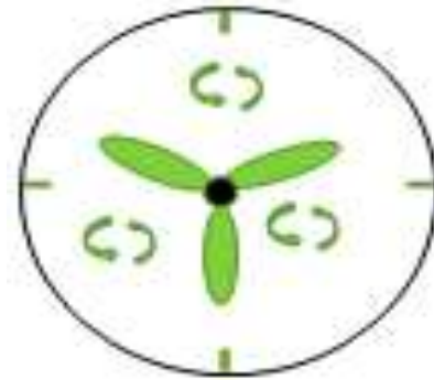
Fig.3 (b). Biogas plant with impeller top view inside digester
