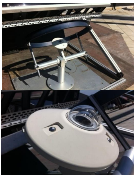
Fig. 4: The two pyranometers for measuring the global and diffuse irradiation, mounted in the collector plane
