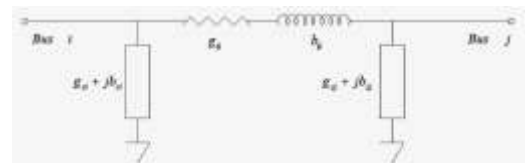
Fig. 1 Pi model of the transmission line [1]
