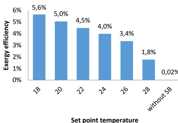
**Fig. 5** Annual exergy efficiency of the case study commercial greenhouse integrated with solar blind system for various set point temperatures
