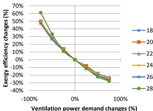
Fig. 9 rate of exergy efficiency changes with ventilation power demand changes for various set point temperatures
