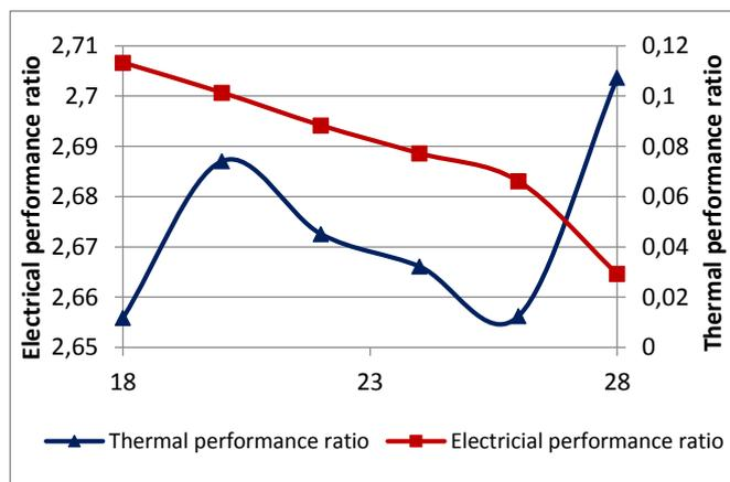
**Fig. 4** Thermal and electrical performance ratio for the commercial greenhouse integrated with solar blind system
