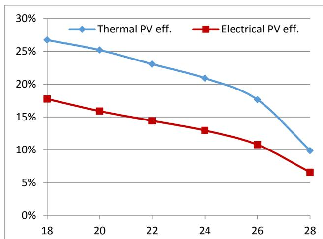
**Fig. 3** Thermal and electrical efficiencies of solar blind system for various set point temperatures
