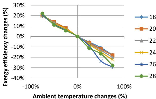
Fig. 10 rate of exergy efficiency changes with ambient temperature changes for various set point temperatures
