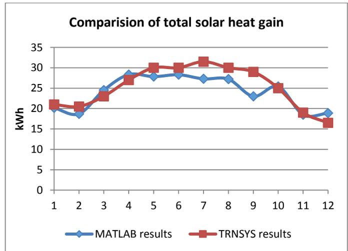
Fig. 2 Comparison of solar useful heat gains
