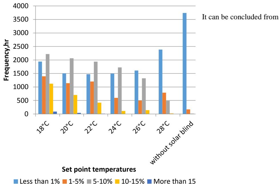
**Fig. 7** Frequency of exergy efficiency for various set point temperatures with comparison with conventional greenhouse without solar blind system
