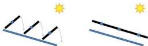
**Fig. 1.** The schematic of solar blind system in both non-operative mode (a) and operative mode (b).
