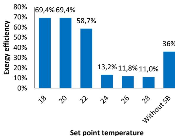
**Fig. 6** maximum possible exergy efficiency (in hourly based calculation) which can be obtained during one whole year for various set point temperatures
