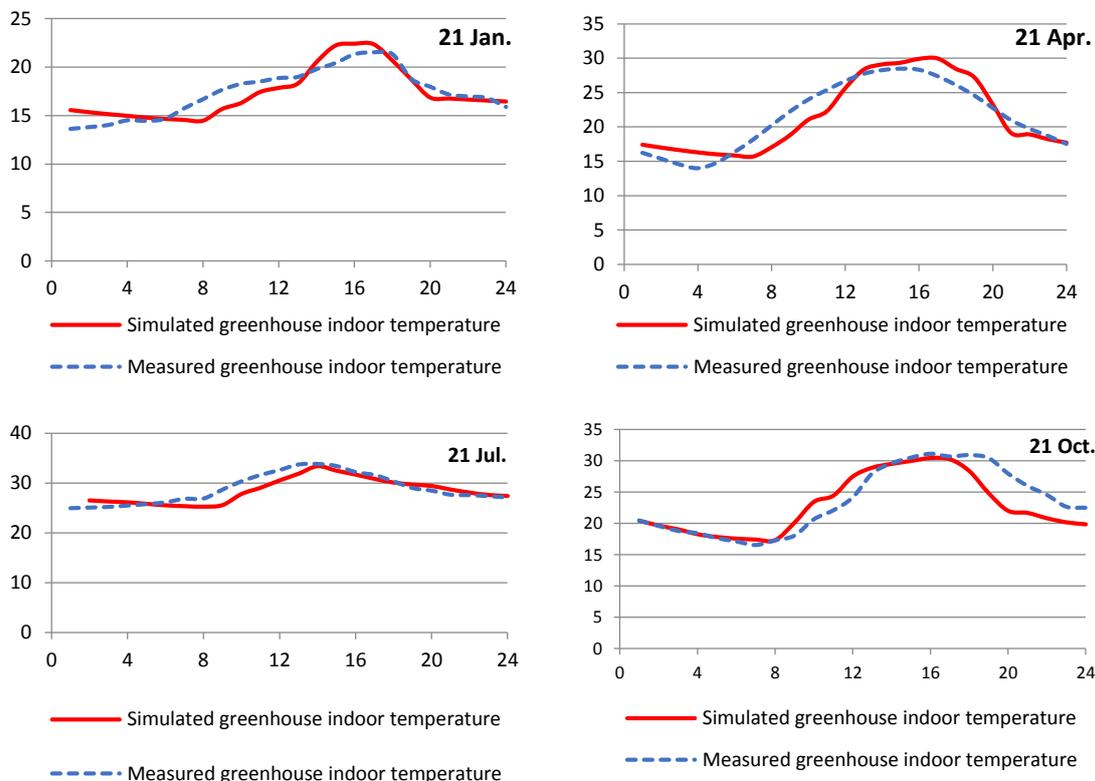
**Fig. 1** Comparison of greenhouse indoor temperature variation for simulated and measure value
