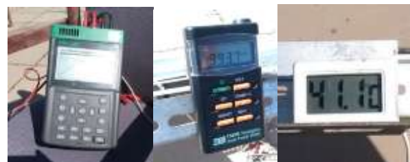
Fig 4. Measuring apparatus from right to left: solar module analyzer, Solar Power meter and digital thermometer.
