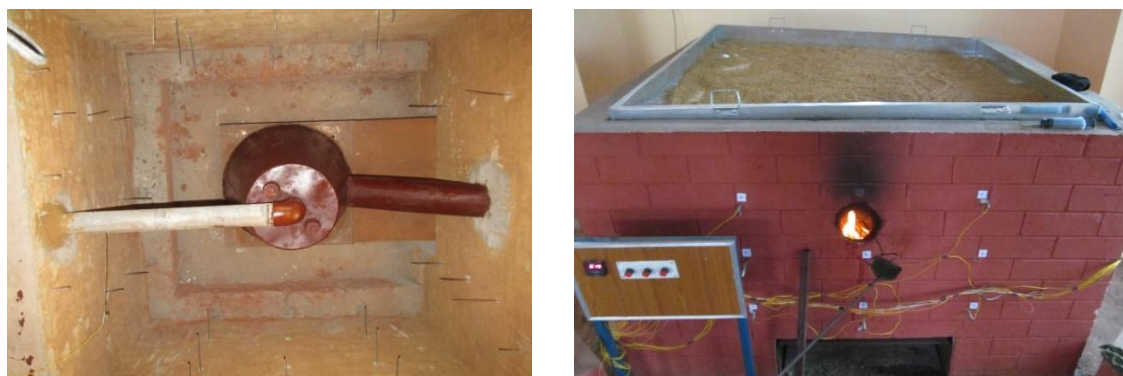
Figure 3. Top view of the Biomass dryer and paddy drying on the dryer.
