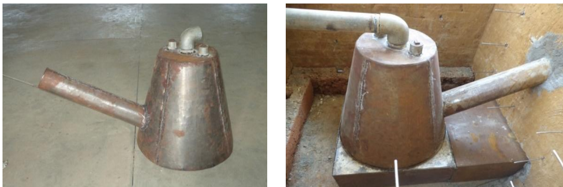
Figure 1. Furnace of the biomass dryer with exhaust pipe.
