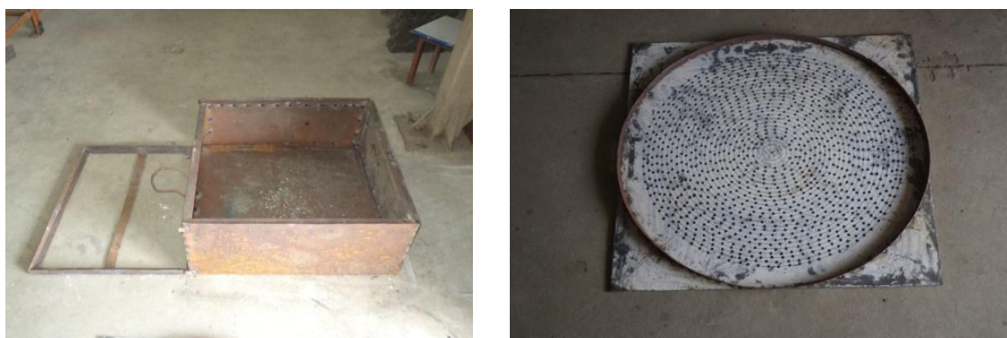
Figure 2. Base of the biomass dryer with ash tray and biomass burning tray.
