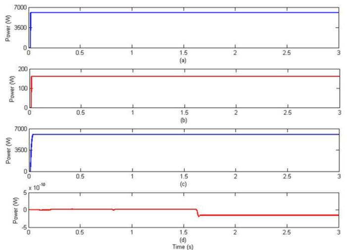
**Fig. 18.** Real and reactive powers (a), (b) without compensation and (c), (d) with compensation
