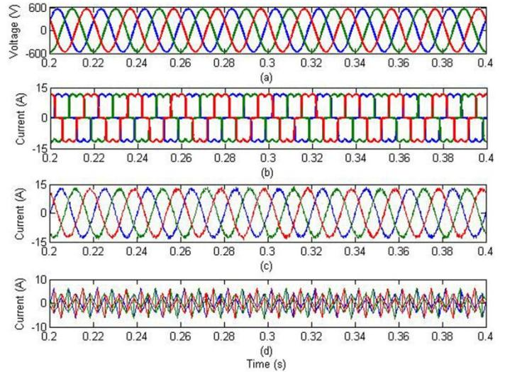
**Fig. 17.** (a) Inverter Voltage (b) current with diode rectifier load (c) current with compensation (d) Compensating current
