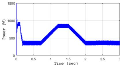
**Fig. 6.** WT output power
