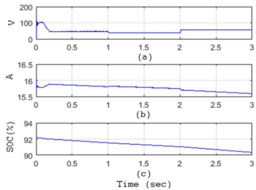
**Fig. 186.** UC (a) voltage (b) current and (c) SOC
