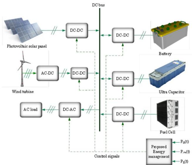
**Fig. 1.** Structure of the HRES with proposed methodology
