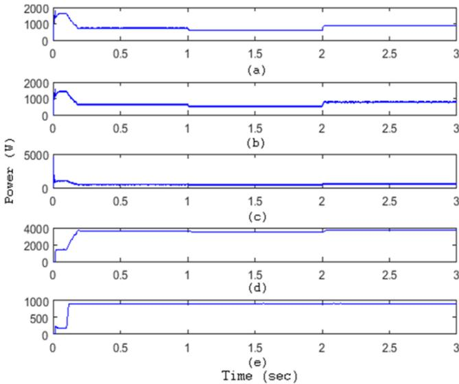
**Fig. 29.** Power produced from (a) UC (b) Battery (c) FC (d) PV and (e) WECS
