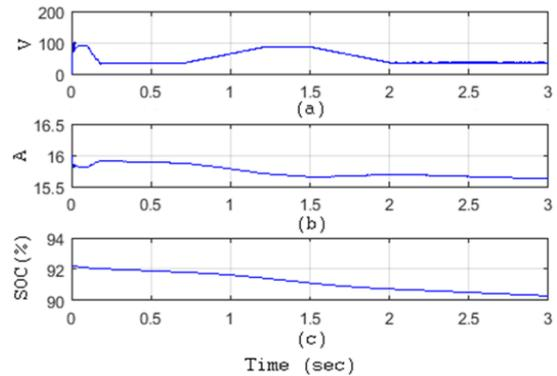
**Fig. 10.** UC (a) voltage (b) current (c) SOC
