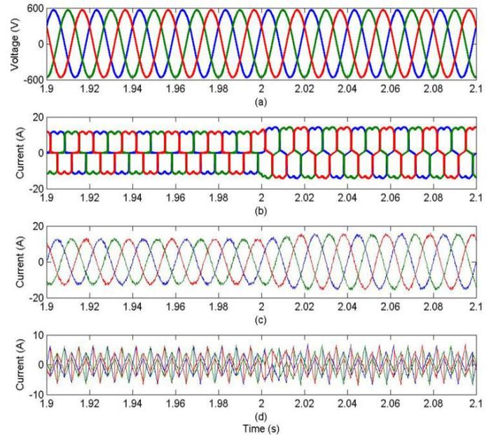
**Fig. 31.** (a) Inverter Voltage (b) current with diode rectifier load (c) current with compensation (d) Compensating current
