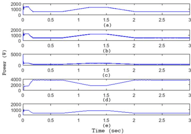
**Fig. 13.** Power produced from (a) UC (b) Battery (c) FC (d) PV and (e) WECS
