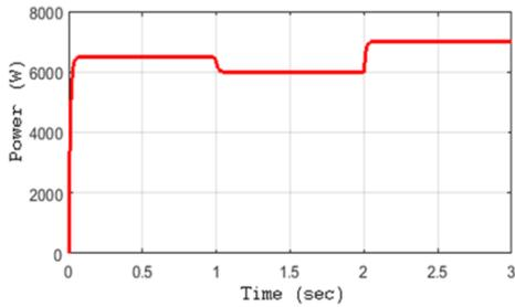
**Fig. 159.** Load demand of the second test case
