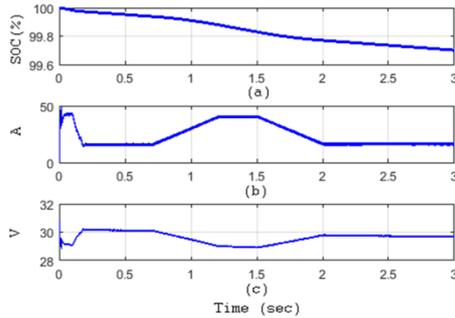
**Fig. 12.** Battery (a) SOC (b) current (c) voltage
