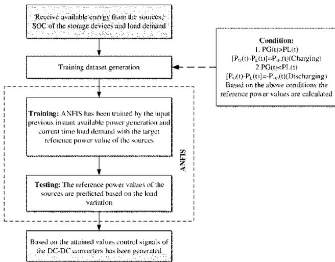
Fig. 2. Structure of the proposed energy management
