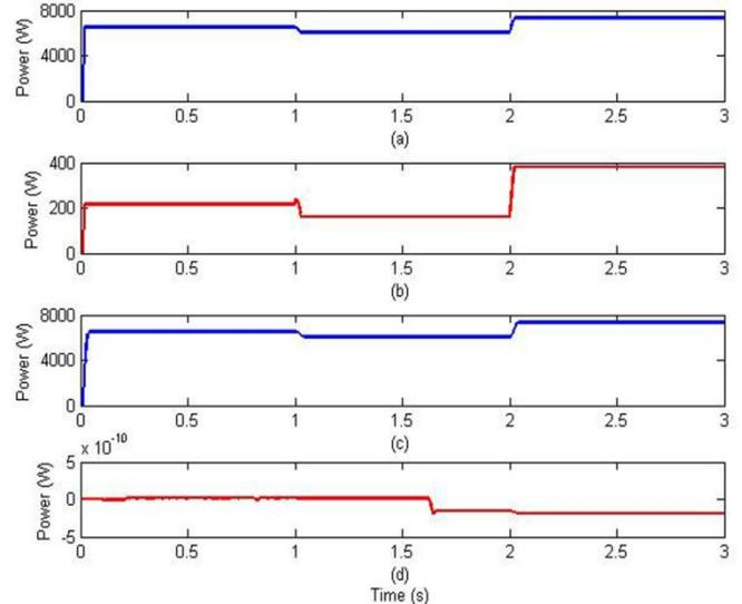
**Fig. 32.** Real and reactive powers (a), (b) without compensation and (c), (d) with compensation
