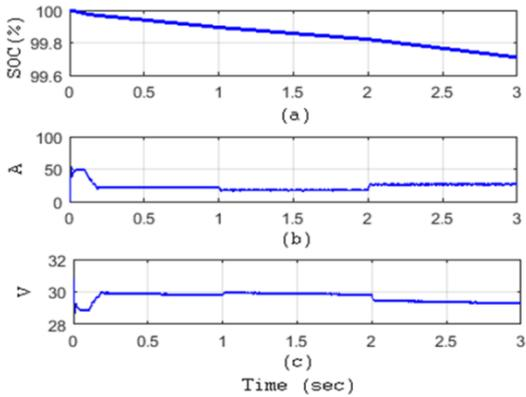
**Fig. 28.** Battery (a) SOC (b) current (c) voltage
