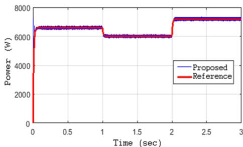
**Fig. 30.** Total power generation with load power reference
