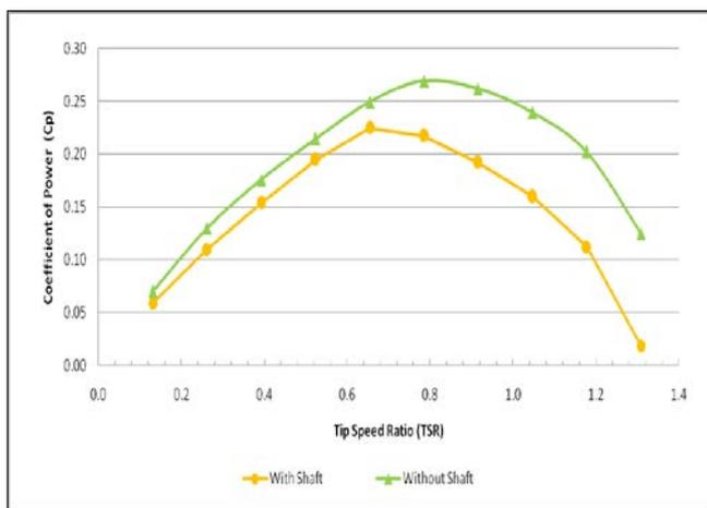
**Fig. 7** Comparison Coefficient of Power ( $C_p$ ) vs  $TSR$ , combined blade rotors without and with shaft.
