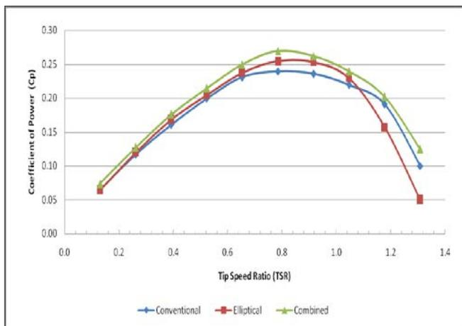
**Fig. 4.** Comparison Coefficient of Power (Cp) vs TSR, conventional, elliptical and combined blade rotors.
