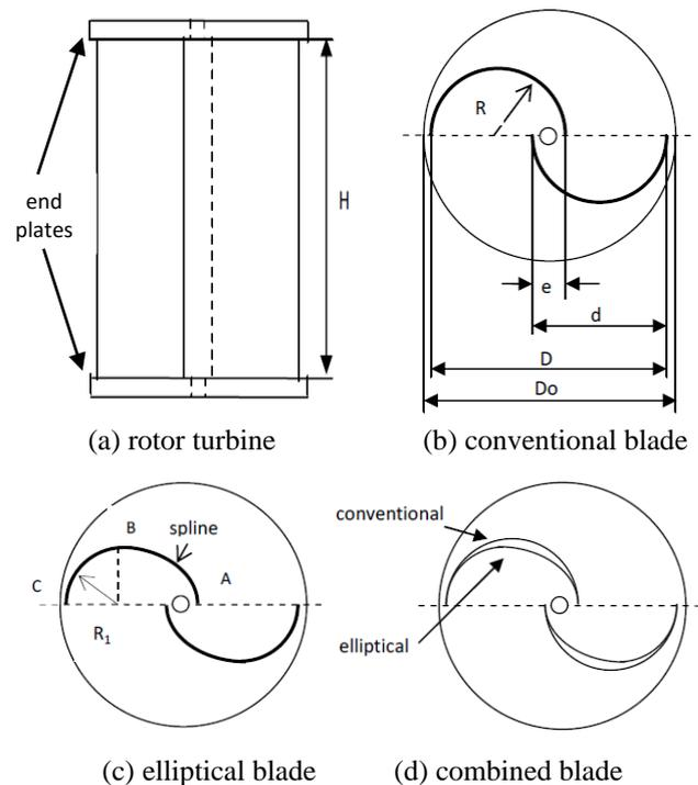
**Fig. 1.** Dimension model of rotor blade turbine Savonius.
