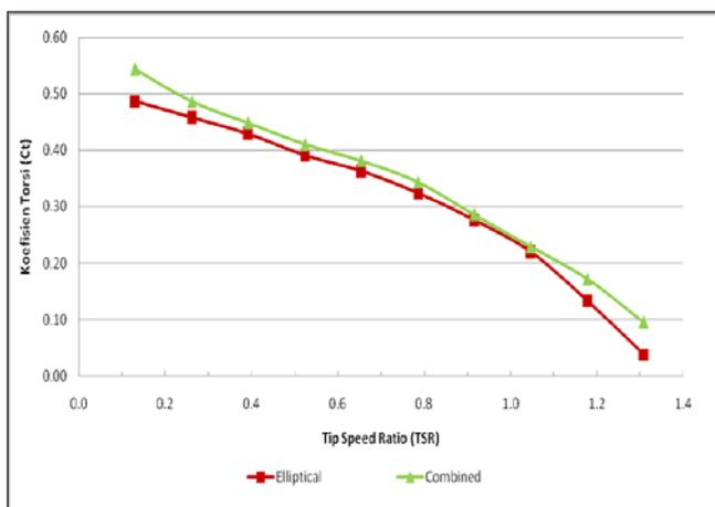
**Fig. 6.** Comparison Coefficient of Torque (Ct) vs TSR, elliptical and combined blade rotors.
