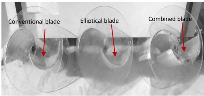
**Fig. 2.** Prototypes blade rotor conventional, elliptical and combined blade with end plates.
