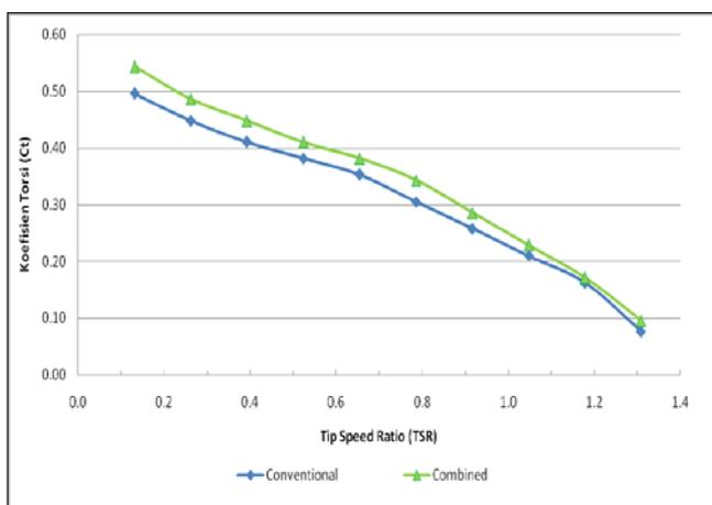
**Fig. 5.** Comparison Coefficient of Torque (Ct) vs TSR, conventional and combined blade rotors.
