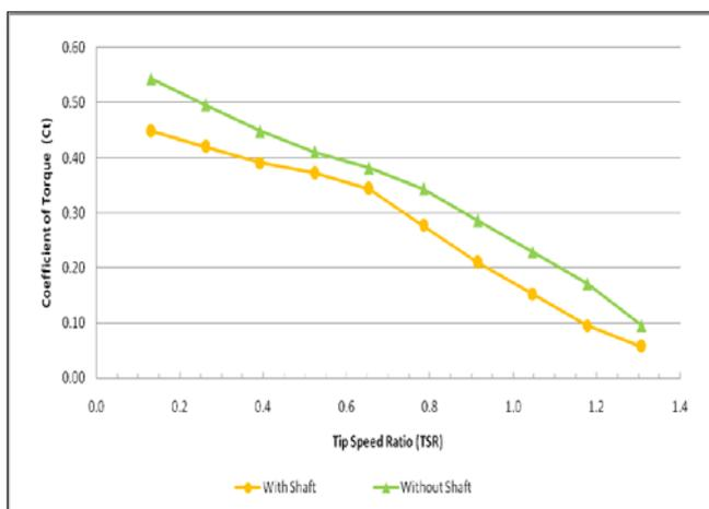
**Fig. 8** Comparison Coefficient of Torque ( $C_t$ ) vs  $TSR$ , combined blade rotors without and with shaft.
