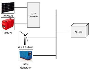
Fig 7. Hybrid system model based on input sources.
