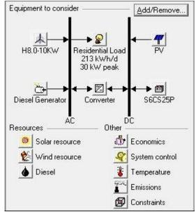
Fig 11. Schematic diagram of PV/Wind/Diesel/Battery system.
