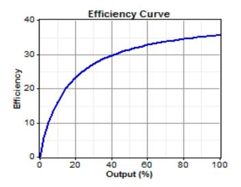
Fig 5. Fuel efficiency curve of diesel generator.
