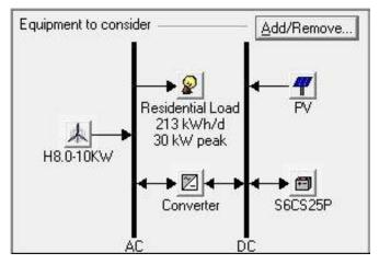
Fig 8. Schematic diagram of PV/Wind/Battery system.
