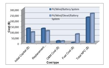
Fig 14. Cost comparison of the two hybrid systems.
