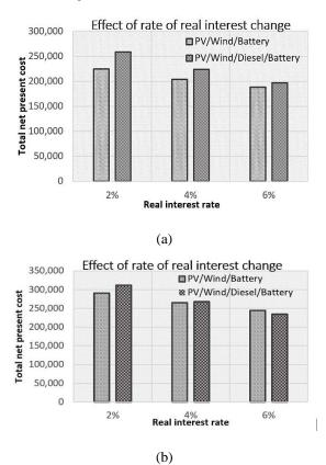
Fig 13. Effect of real rate of interest change for (a) load 213 kWh/day, (b) load 277 kWh/day
