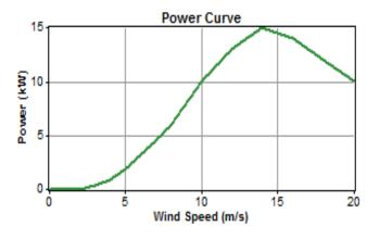
Fig 6. Wind speed vs power curve of wind turbine.
