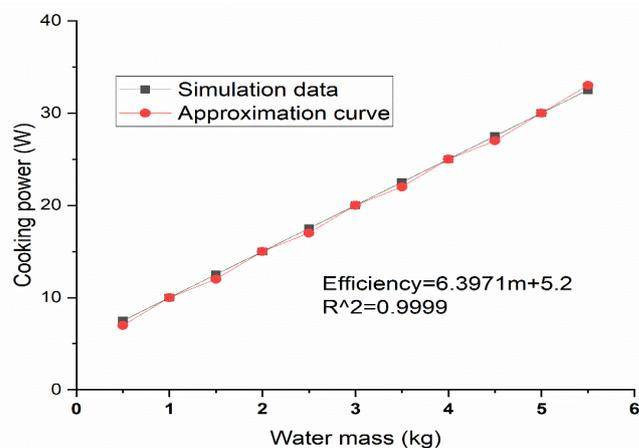
**Fig 9.** standard firing output as a function of the mass of water in the solar cooker container.
