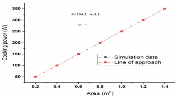
**Fig 4.** Solar cooker collector area thermal performance
