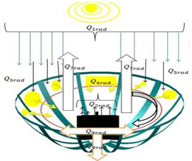
**Fig 2.** Solar cooker heat fluxes by radiation and convection
