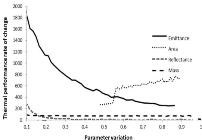
**Fig 11.** Thermal performance change as a result of design variables for solar cookstoves
