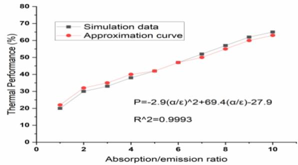
**Fig 6.** Emittance-to-absorbance ratio of thermal performance
