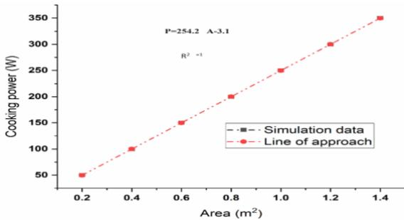
**Fig 3.** Standard firing output.
