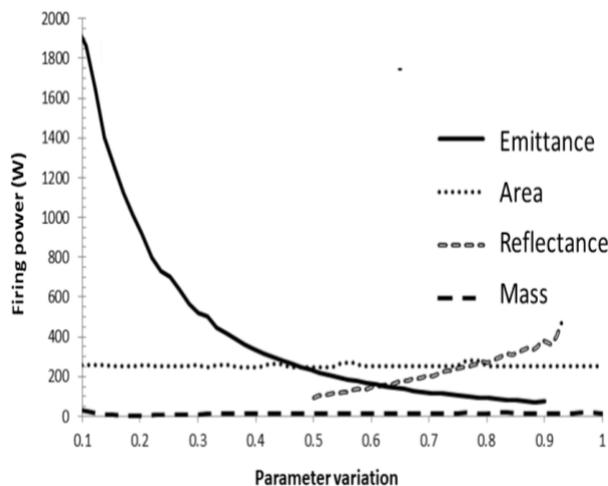
**Fig 10.** The ratio of the standard firing output to the design variables of the solar cooker
