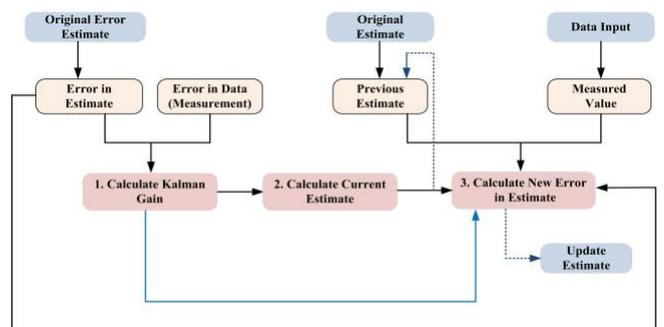
Fig. 3. Kalman Filtering Principle
