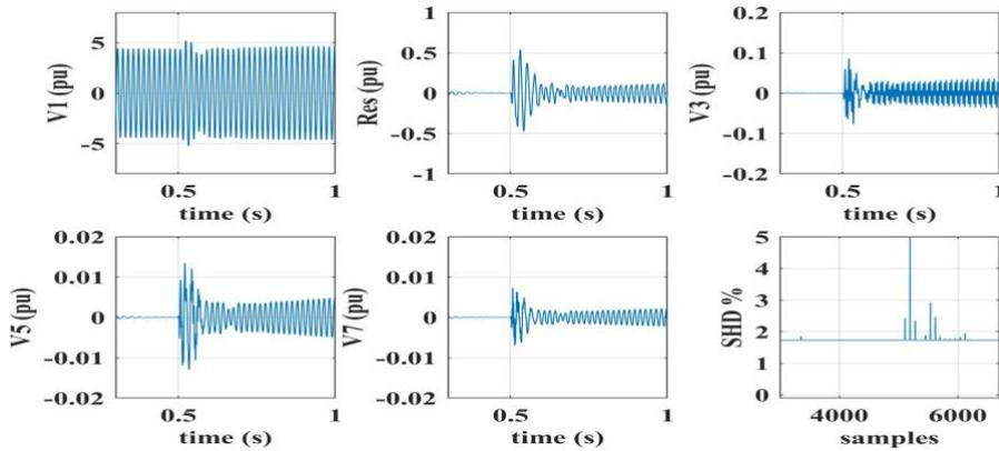
**Fig. 9.** Islanding detection in an imbalanced condition
