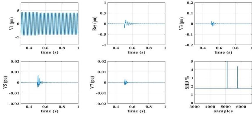
**Fig. 8.** Islanding detection with a parallel RLC load PV
