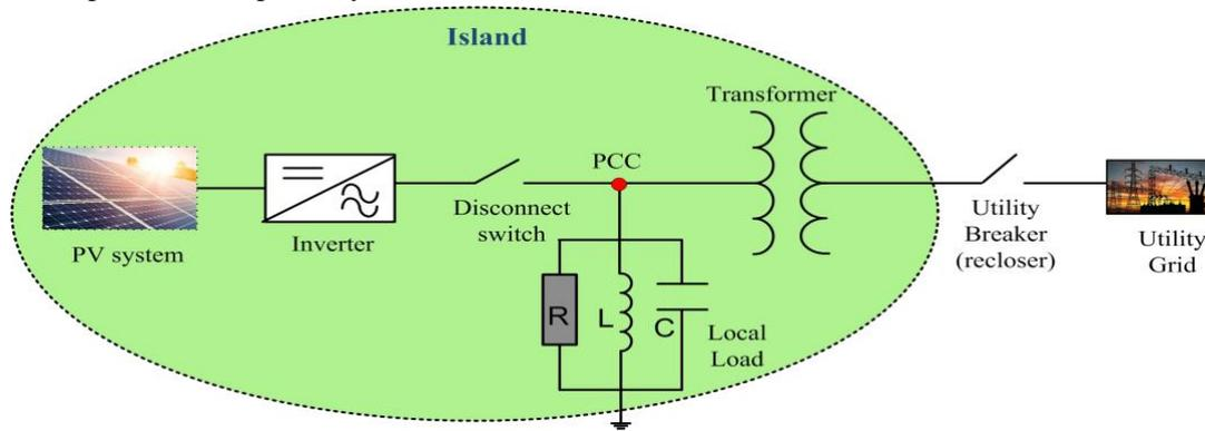
**Fig. 1.** Islanding formation in DG integrated-based power system
