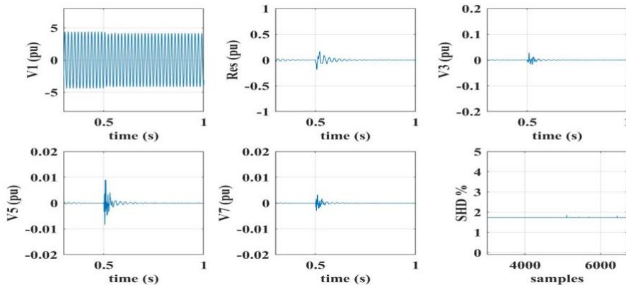
**Fig. 10.** Islanding detection in balanced condition
