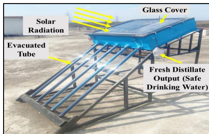
Fig. 2: Description of the equipment and arrangement used for the experiment.
