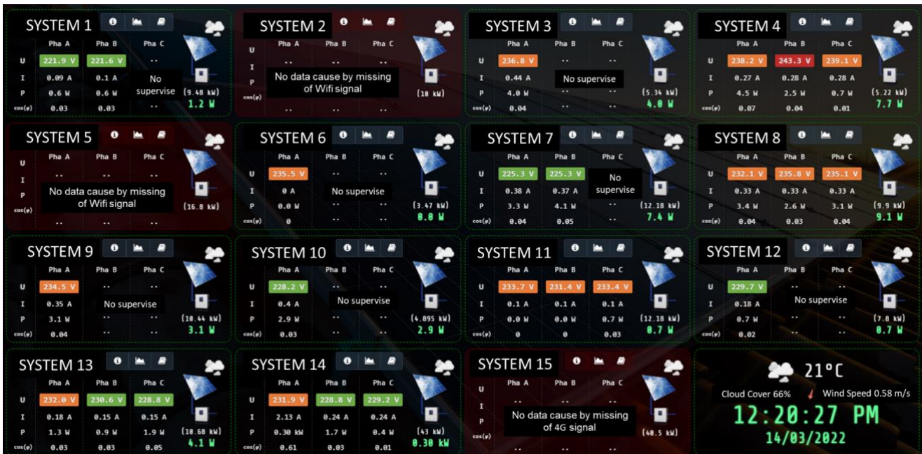
b. Monitoring interface of multiple rooftop solar power stations
