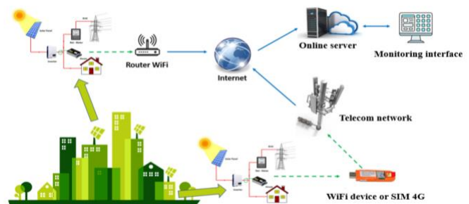
Fig. 1. Working principles of the monitoring and data acquisition system
