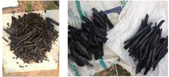
Fig 8. Charcoal obtained from the vertical charcoal kiln with a double layer to prevent heat loss
