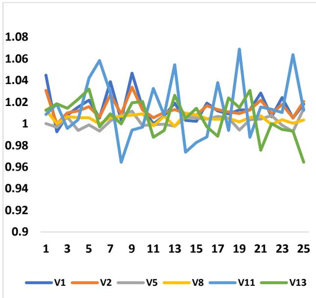
**Fig. 2.** Optimal settings of generator bus voltages for all scenarios in multi objective case with solar and wind power
