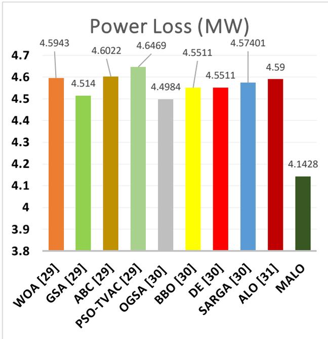
Fig. 1. Power loss values for different optimization techniques for ORPD
