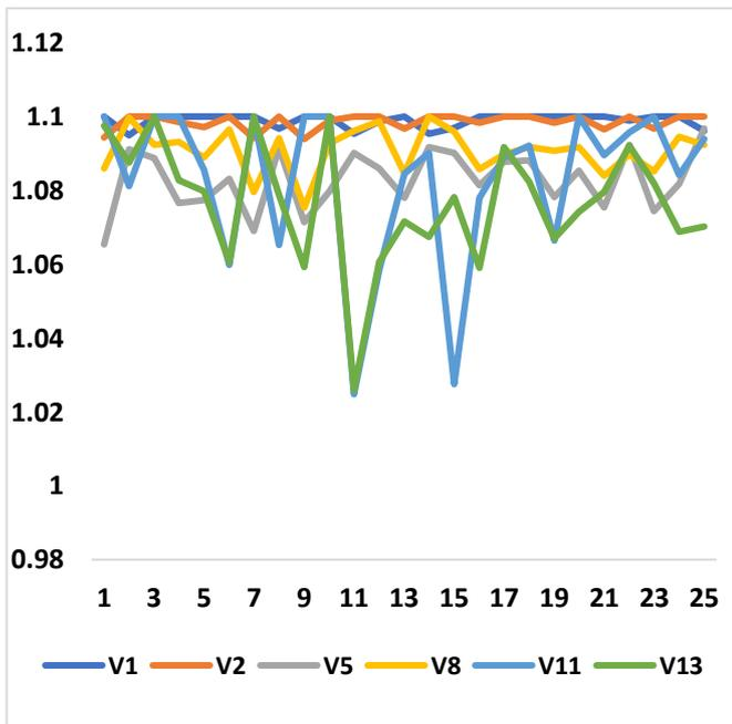
**Fig. 3.** Optimal settings of generator bus voltages for all scenarios in power loss minimization case with solar and wind power
