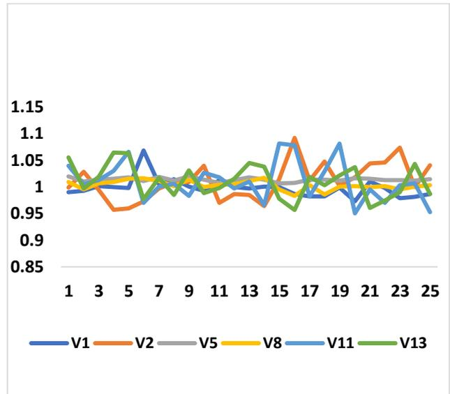
**Fig. 4.** Optimal settings of generator bus voltages for all scenarios in voltage deviation minimization case with solar and wind power
