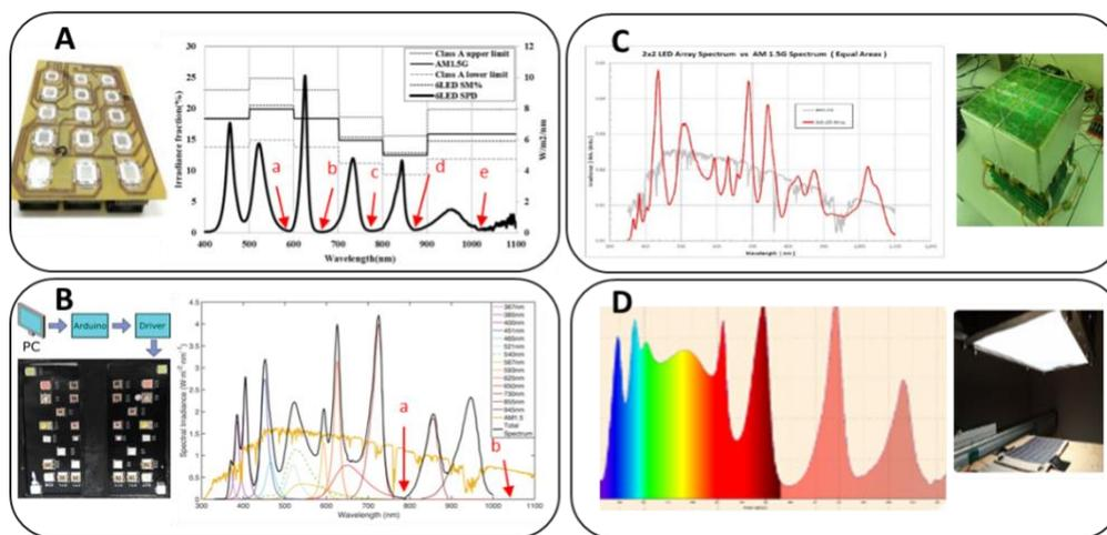
**Fig. 2.** The example of the LED light sources and spectrum coverage and uncoverage of LED spectrum from the reviewed (a) SPD of 6 LEDs show uncoverage at point a, b, c, d, and e [3], (b) SPD of 14 LEDs show uncoverage at point a, b [61], (c) Coverage spectrum from 23 LEDs [24], and (d) 10 LEDs [63].
