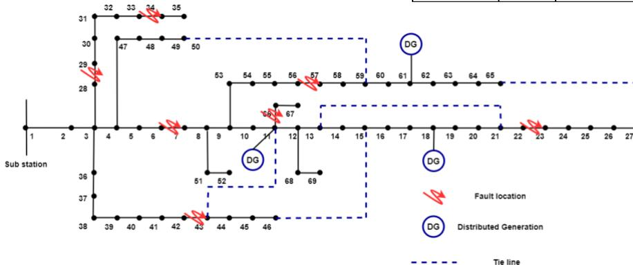
Fig. 8. IEEE 69 bus Distribution test system
