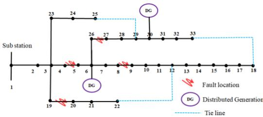
**Fig. 4.** IEEE 33 bus Distribution test system
