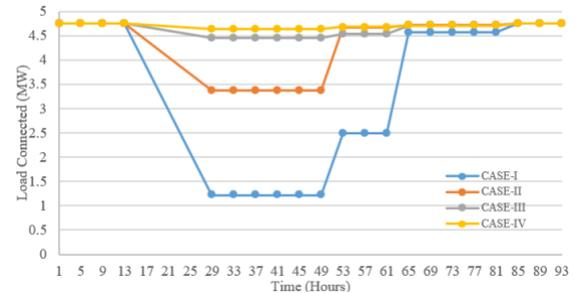
**Fig. 10.** Operational trapezoids for IEEE 69 bus distribution system under 125% overloading conditions
