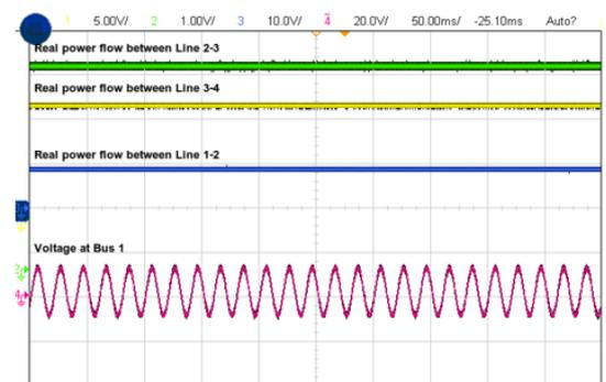
**Fig. 17.** Results showing after adding DG and Tielines
