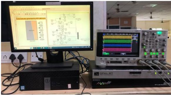
**Fig. 12** Hardware set up OPAL-RT OP4510
