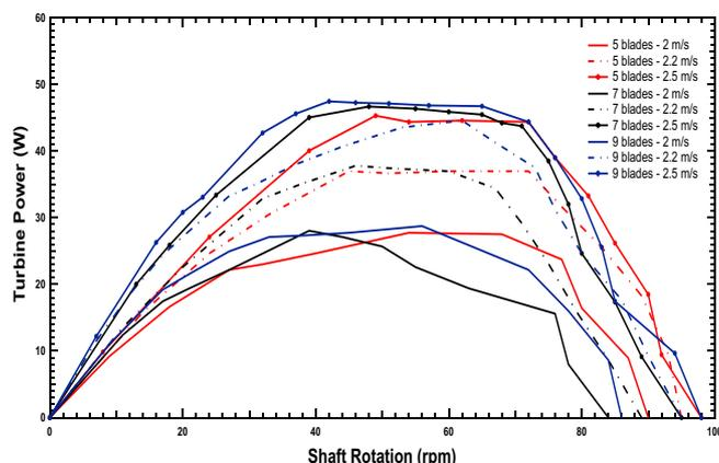
Fig. 8. Turbine power versus shaft rotation for 5, 7, and 9 blades.
