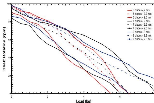
Fig. 6. Shaft rotation versus load for 5, 7, and 9 blades.
