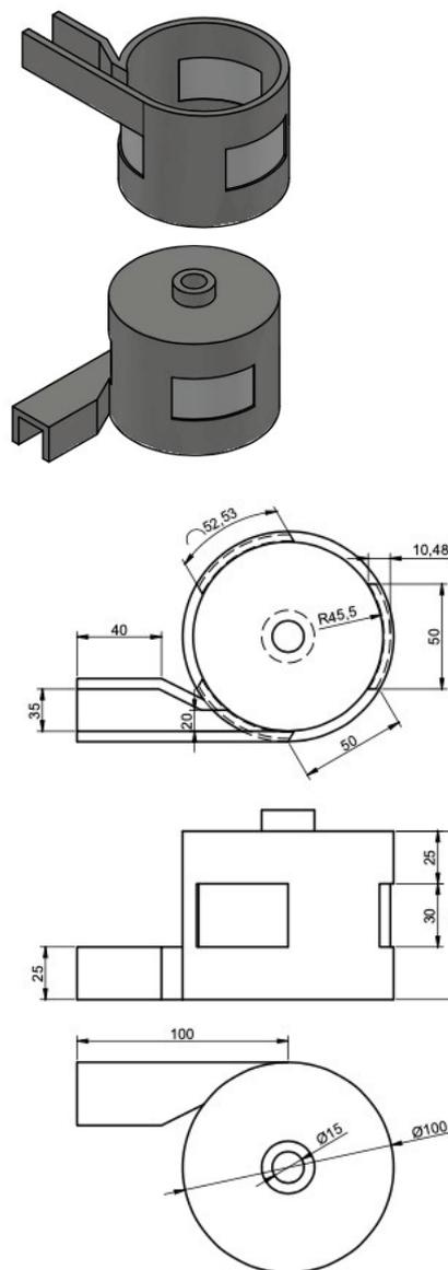
**Fig. 2.** Design of basin and intake tunnel.
