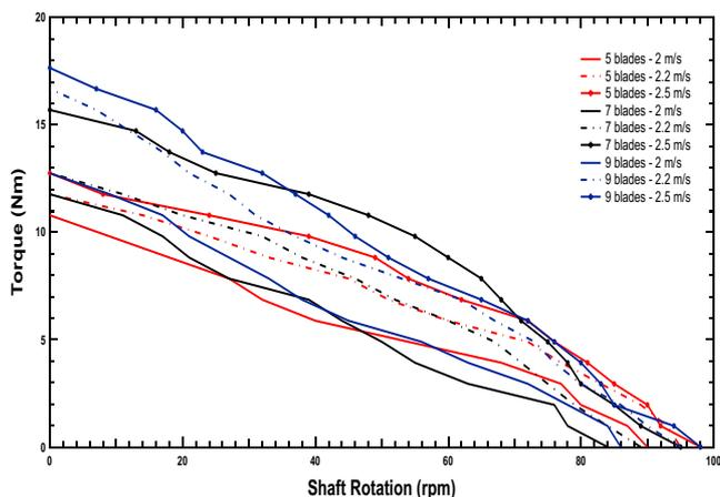
Fig. 7. Torque versus shaft rotation for 5, 7, and 9 blades.
