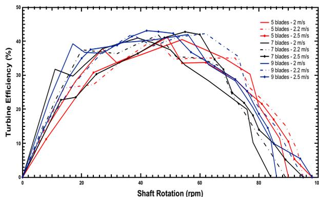
Fig. 9. Turbine efficiency versus shaft rotation for 5, 7, and 9 blades.
