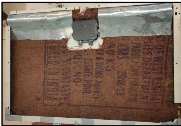
Fig. 5. Rear surface of PV module covered with burlap
