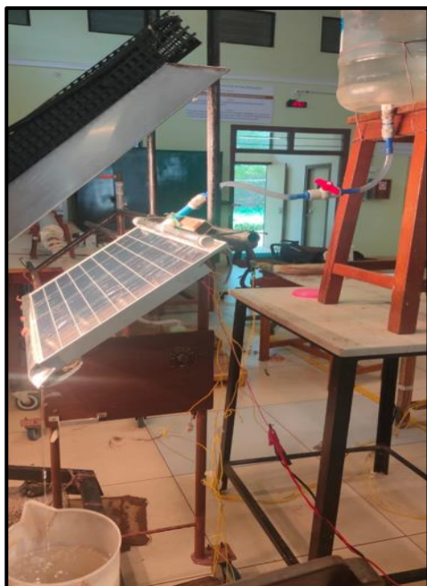
Fig. 6. PV front cooling arrangement
