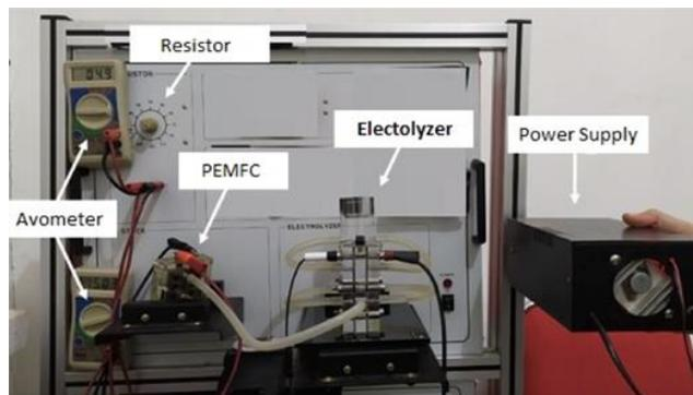
Fig. 2. MEA testing equipment on PEMFC
