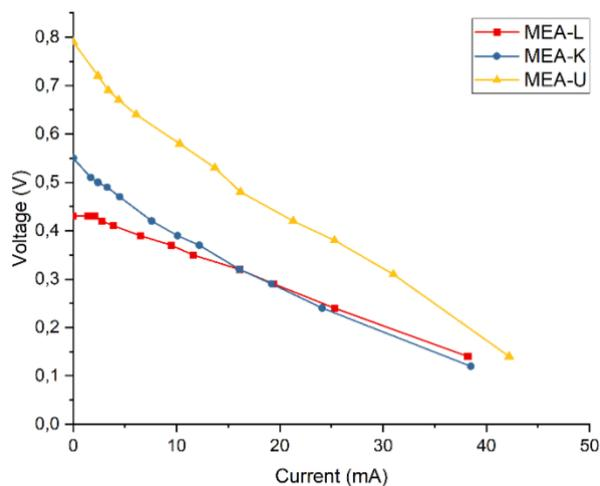
Fig. 4. Comparison graph of voltage-to-current between MEA-L, MEA-K, and MEA-U
