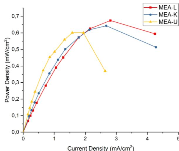
Fig. 5. Comparison graph of power density-to-current density of MEA-L, MEA-K, and MEA-U
