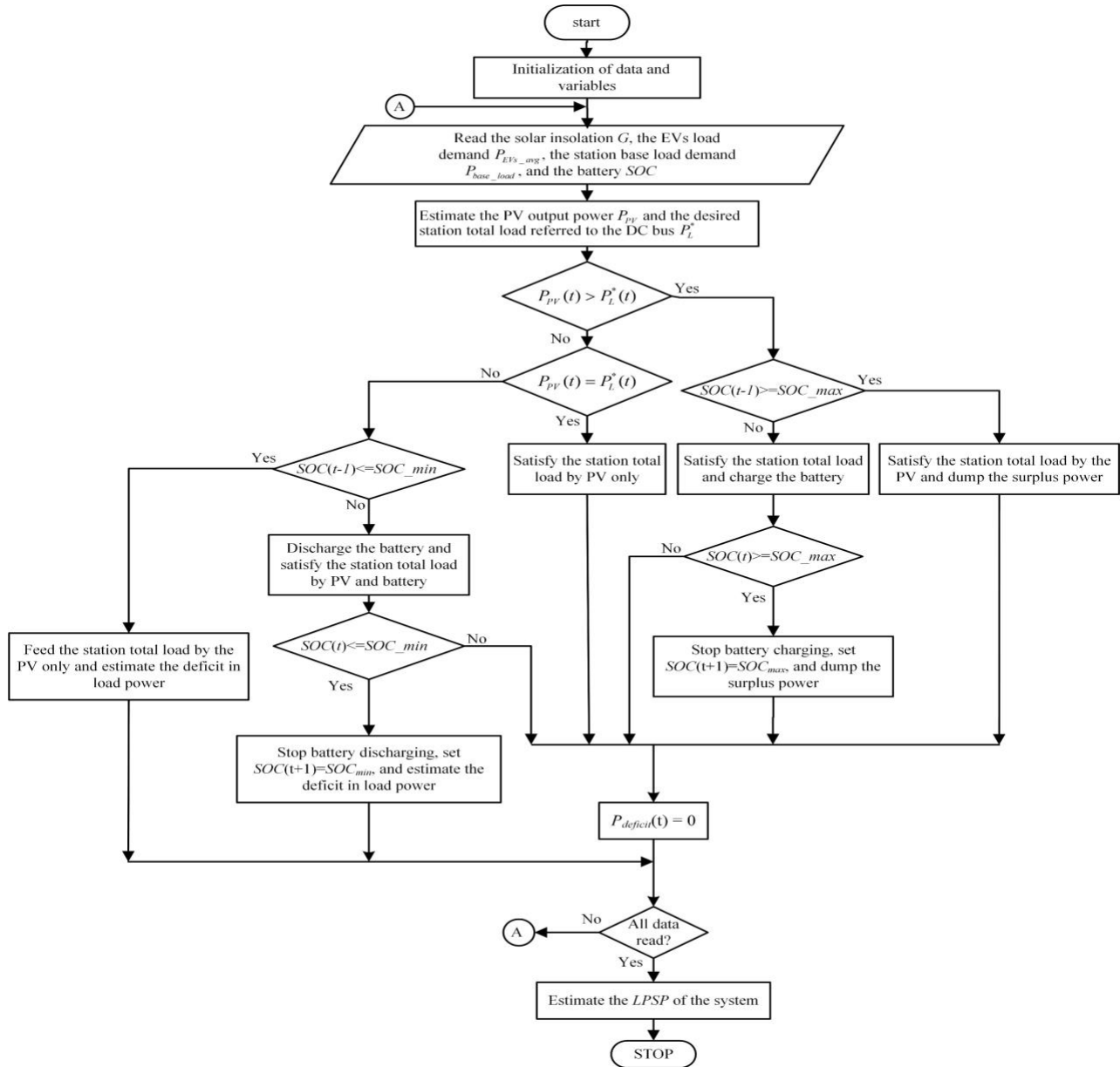
Fig. 5. Proposed energy management of the PV-battery stand-alone FCSEVs.
