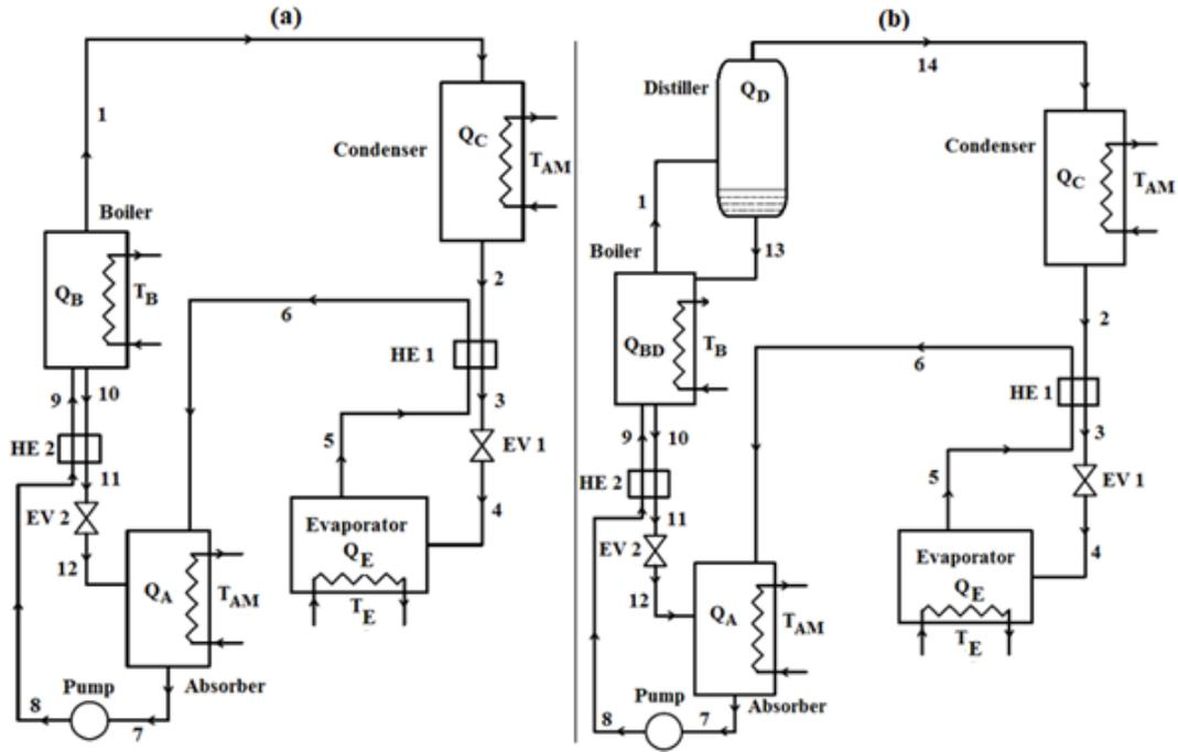
**Fig. 1.** Schematic representing of single-stage absorption refrigeration system: (a) without distiller mechanism; (b) with distiller mechanism.
