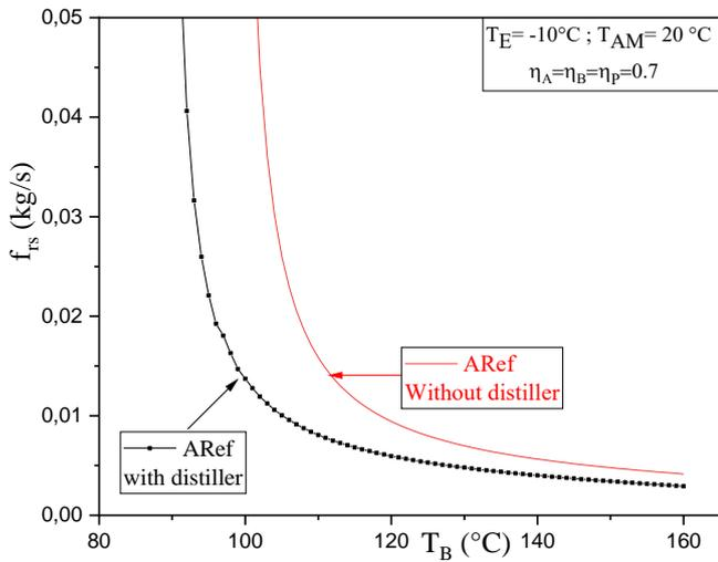
**Fig. 3.** Influence of thermal distillation process on the flow rate of rich solution coming out from the absorber.
