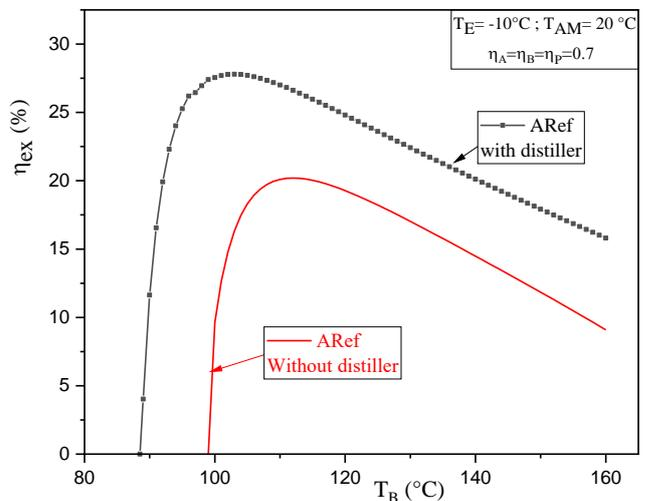
Fig. 6. Evolution of the exergy efficiency for the two absorption refrigerators analyzed (with and without distiller).
