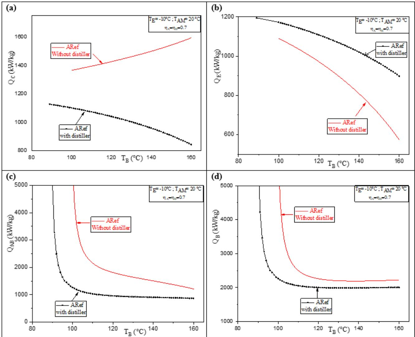
Fig. 5. Effect of distillation on the different quantities of heat exchanged by the absorption system's heat exchangers.
