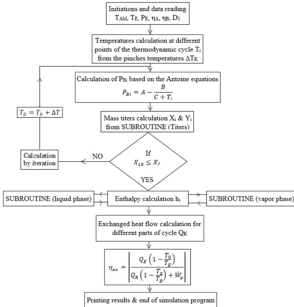
Fig. 2. Flowchart representing the different simulation steps.
