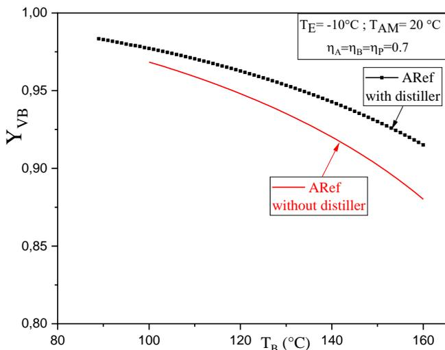
**Fig. 4.** Influence of thermal processes on the vapor concentration coming out from the boiler.
