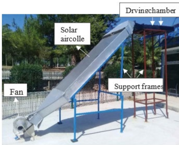
Fig. 3 Mixed mode type solar dryer
