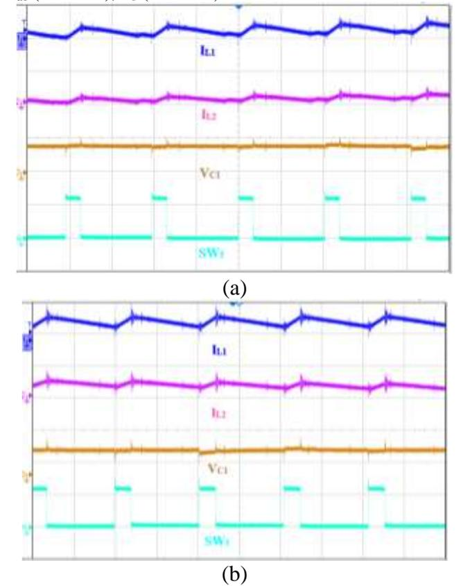
**Fig. 15.** Experimental results of  $I_{L1}$ ,  $I_{L2}$ ,  $V_{C1}$ , and  $SW_5$  (a)  $D=0.1$ ,  $I_{L1}$  (1 A/div),  $I_{L2}$  (1 A/div),  $V_{C1}$  (40 V/div),  $SW_5$  (10 V/div) (b)  $D=0.2$ ,  $I_{L1}$  (2 A/div),  $I_{L2}$  (2 A/div),  $V_{C1}$  (50 V/div),  $SW_5$  (10 V/div).
