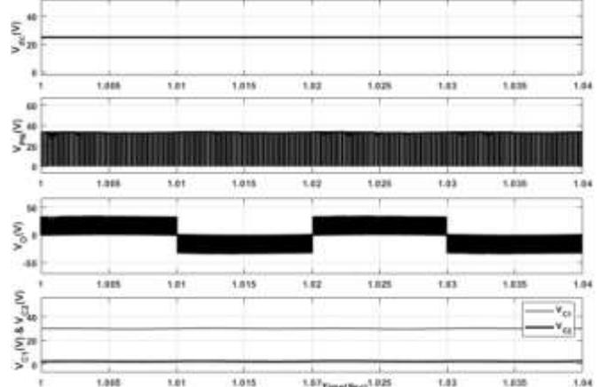
Fig. 9. Waveform of  $V_{dc}$ ,  $V_{PN}$ ,  $V_o$ ,  $V_{C1}$  and  $V_{C2}$  of EBASC-ZSI topology with  $D=.1$ .
