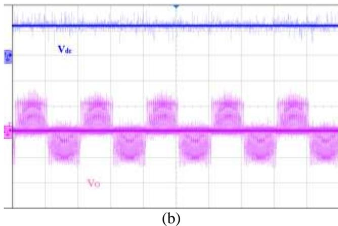
**Fig. 14.** Experimental results of  $V_{dc}$  and  $V_o$  of EBASC-ZSI topology (a) at  $D=0.1$ ,  $V_{dc}$  (20 V/div),  $V_o$  (20 V/div) (b)  $D=0.2$ ,  $V_{dc}$  (20 V/div),  $V_o$  (50 V/div).
