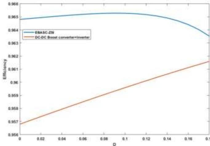
Fig. 8. Comparison of  $D$  verses efficiency of EBASC-ZSI topology and DC-DC boost converter at  $D=.1$ .
