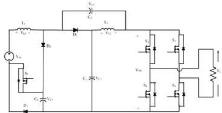
Fig. 3. Schematic diagram of EBASC-ZSI topology.
