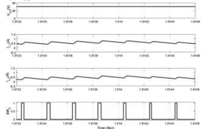
Fig. 10. Waveform of  $V_{C3}$ ,  $I_{L1}$ ,  $I_{L2}$  and  $SW_5$  of EBASC-ZSI topology with  $D=.1$ .
