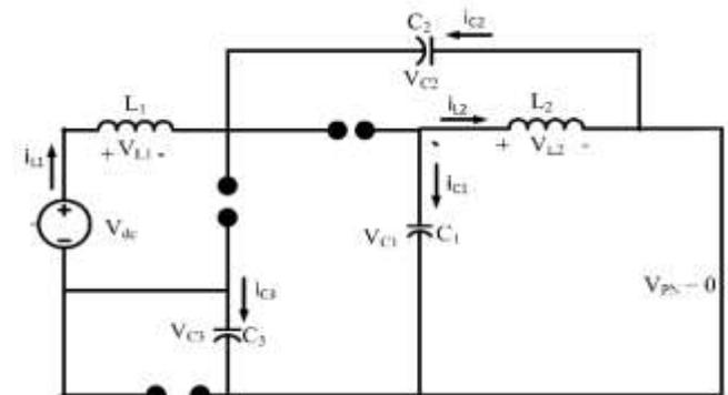
Fig. 4. Schematic diagram of EBASC-ZSI topology in ST state mode.
