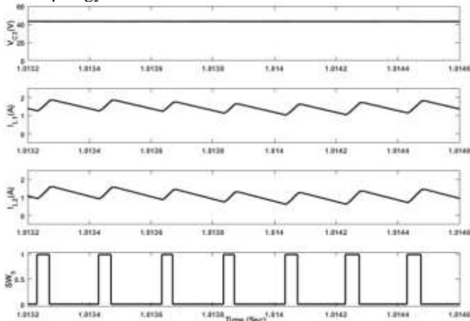
**Fig. 12.** Waveform of  $V_{C3}$ ,  $I_{L1}$ ,  $I_{L2}$  and  $SW_5$  of EBASC-ZSI topology with  $D=0.2$ .
