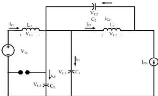
Fig. 5. Schematic diagram of EBASC-ZSI topology in NST state mode.
