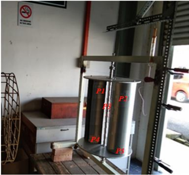
Fig. 13. Uniformity wind test with five points
