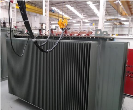
Fig. 3. The experimental setup used to measure losses and short circuit impedance
