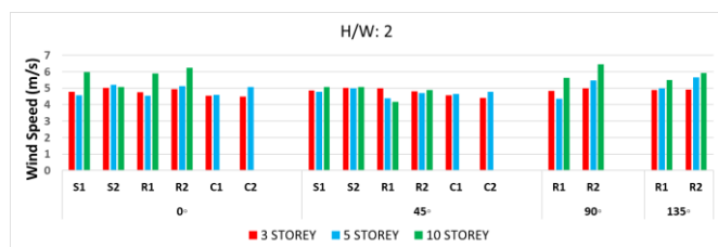
Fig. 10. Wind speed values calculated at z = 14 m (for 3 stories), z = 22 m (for 5 stories), z = 38 m (for 10 stories), for June 21st for a H/W ratio of 2.
