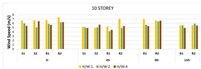
Fig. 11. Wind speed values calculated at z = 14 m (for 3 stories), z = 22 m (for 5 stories), z = 38 m (for 10 stories), for June 21st for a H/W ratio of 4.
