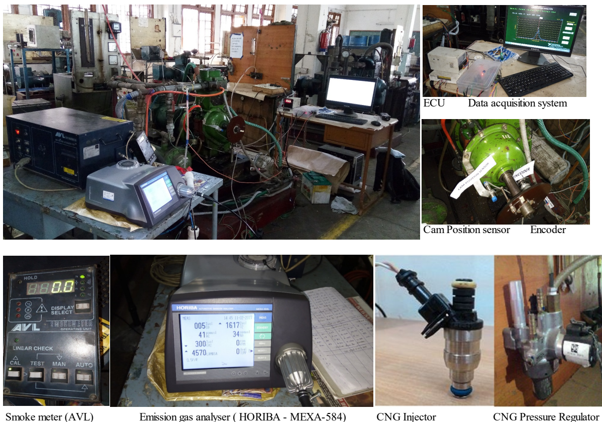
Smoke meter (AVL) Emission gas analyser ( HORIBA - MEXA-584) CNG Injector CNG Pressure Regulator
