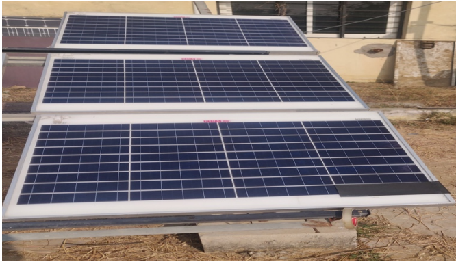
Fig. 4. One cell of the array shaded with 100% strength to mimic cell failure.
